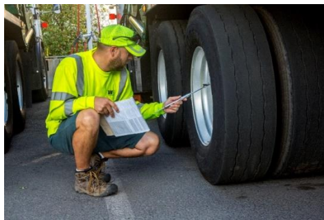
Checking tire pressure
