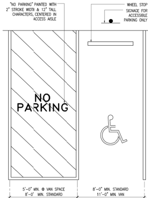
02 ENLARGED TAS PARKING PLAN SCALE 1/4"=1'-0"
