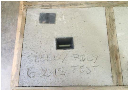
Concrete Block with Polymeric Bar
