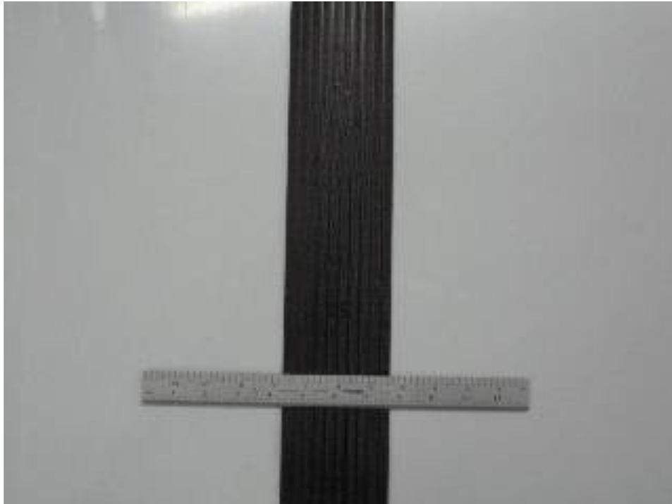
**Figure 1-2. Photo of ParaWeb 50 (machine direction is perpendicular to ruler shown).**
