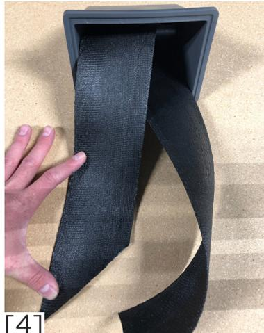
Note: cutting Paraweb strap at angle as shown (image 4) helps reduce friction when inserting strap through box.
