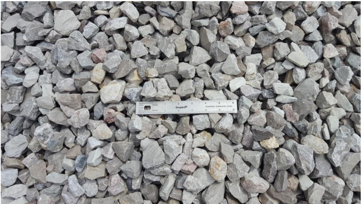
Figure 4-2. Installation damage Type 1 test aggregate.
