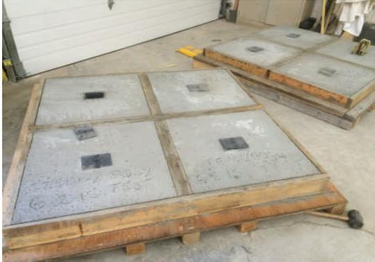
Concrete Blocks as Received (Plywood Lid Removed)
