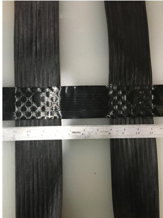
**Figure 1-4. Photo of ParaLink 300 (machine direction is perpendicular to ruler shown).**
