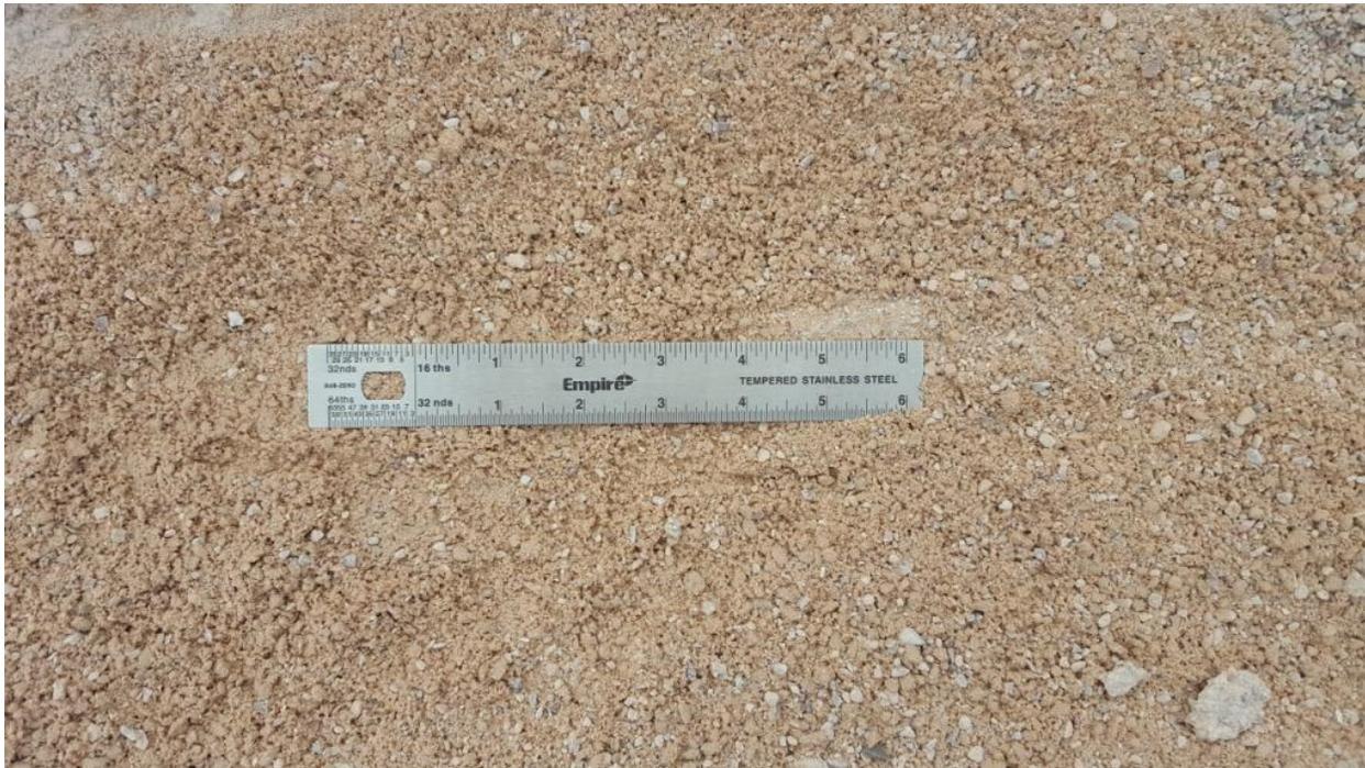
**Figure 4-4. Installation damage Type 3 test aggregate.**
