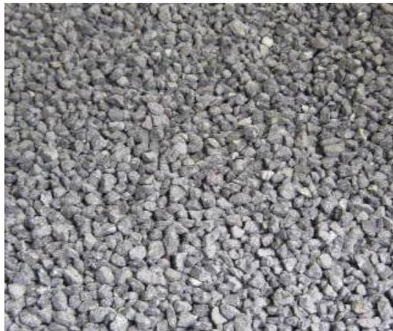
**Figure E-2. ISO/EN 10722, laboratory installation damage aggregate.**
