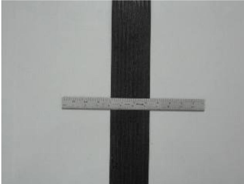
**Figure 1-1. Photo of ParaWeb 30 machine direction is perpendicular to ruler shown).**
