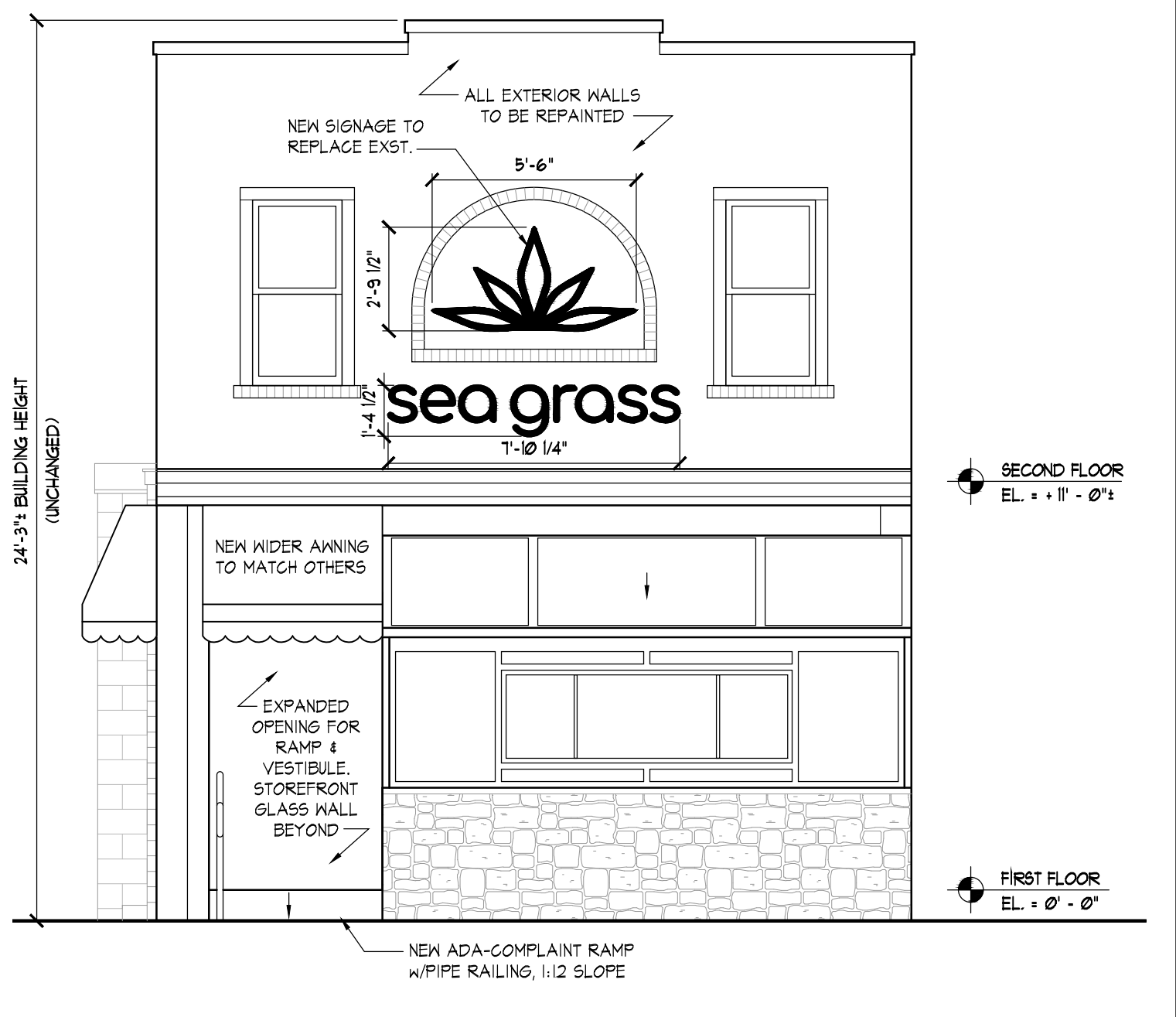
1 FRONT (BAY AVE.) ELEVATION A4 1/4" = 1'-0"
