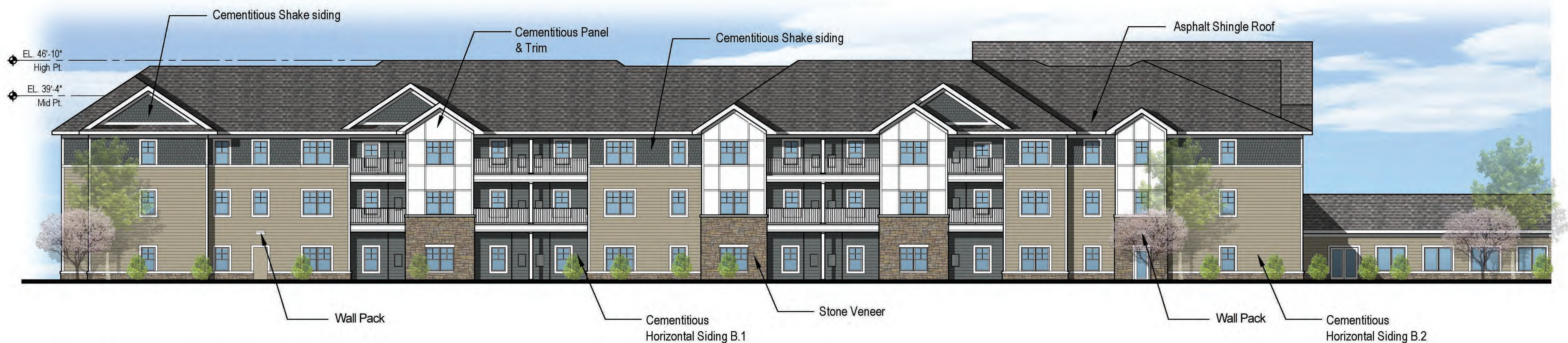
C - WEST ELEVATION- Apartment
