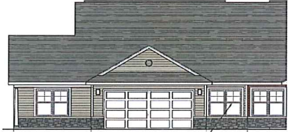
TYPICAL 12:5 PITCH ROOF - INTERNAL UNITS
