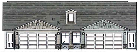
TYPICAL 12:5 PITCH ROOF - INTERNAL UNITS
