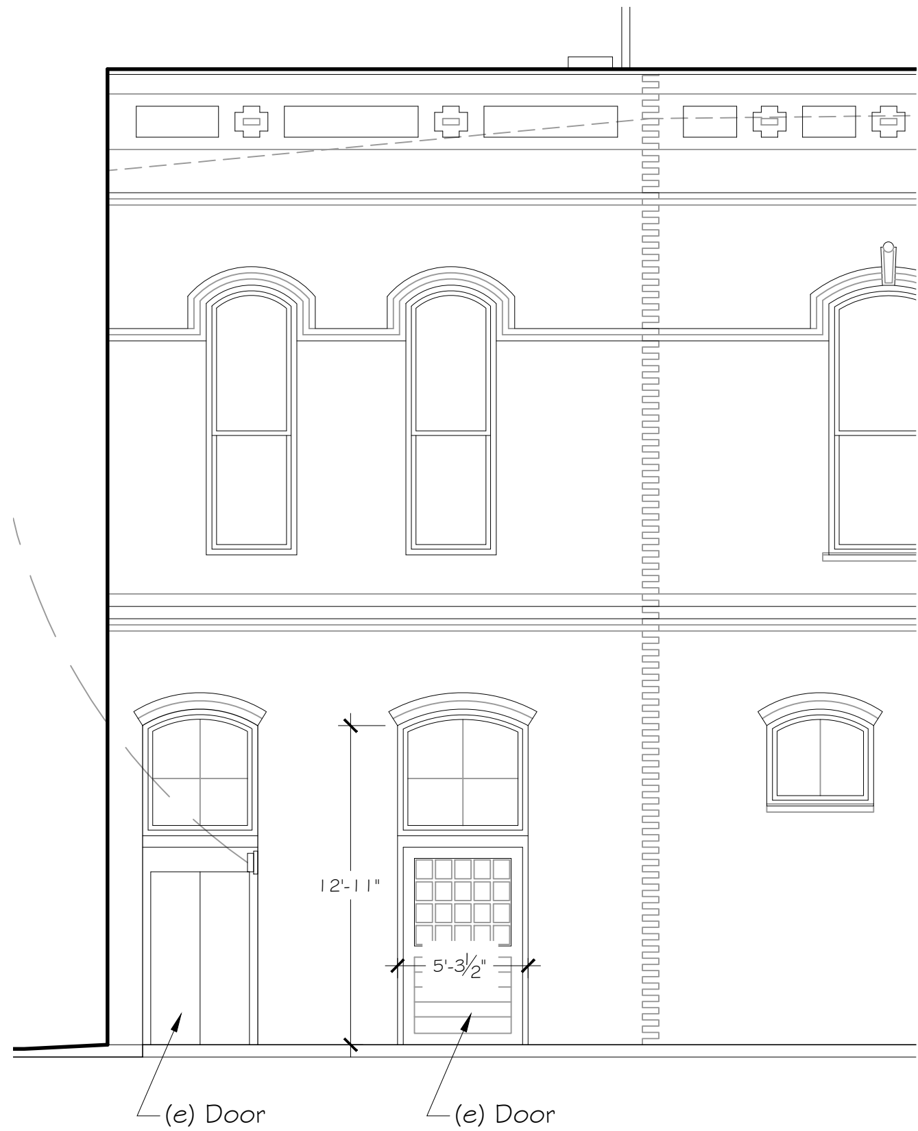
b EXISTING ELEVATION scale: \frac{3}{16}'' = 1' - 0'' when printed on 11x17
