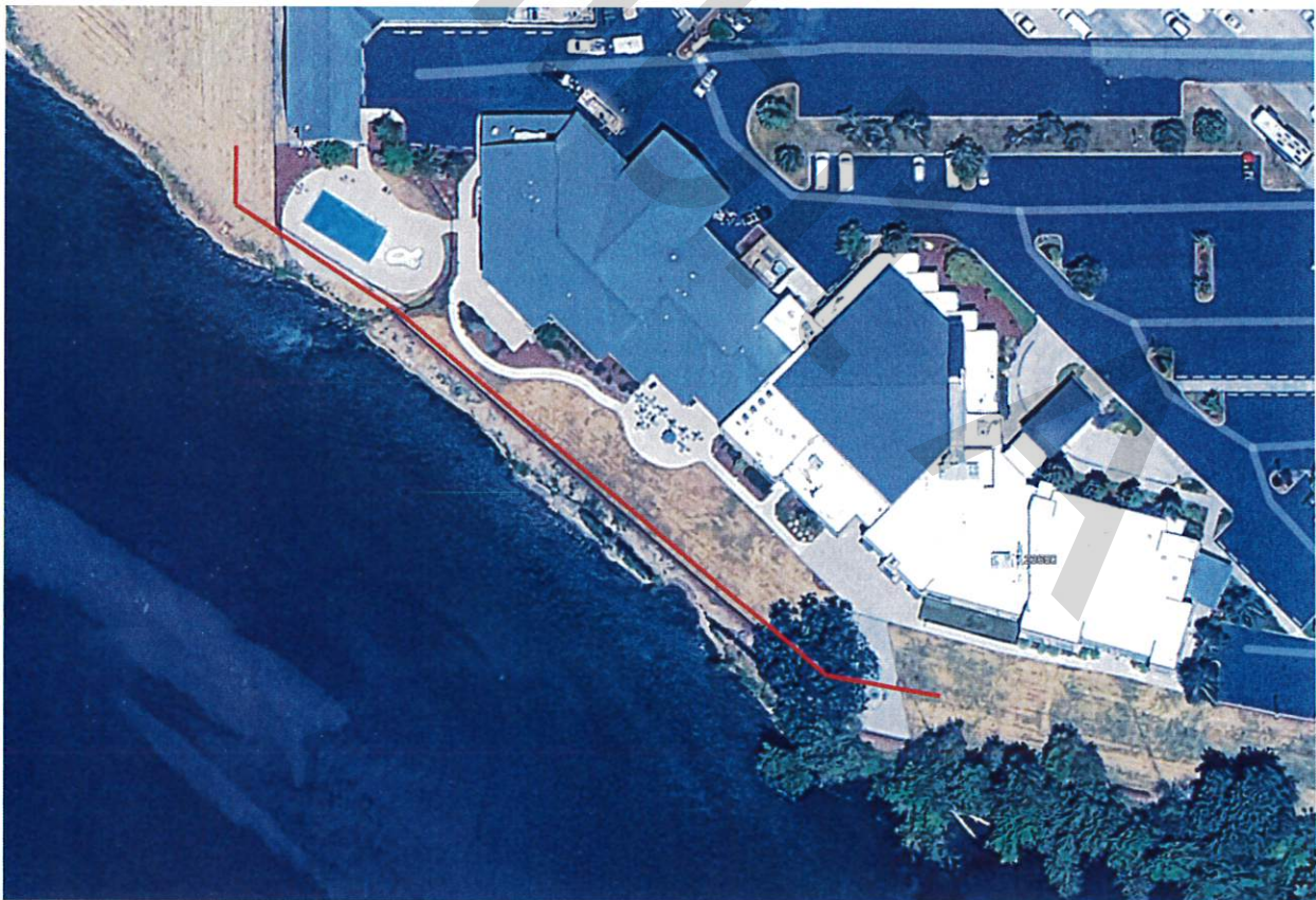
Figure 10: Conceptual sheetpile wall (red lines) approximate location and extents shown relative to the church and eroded bank.
