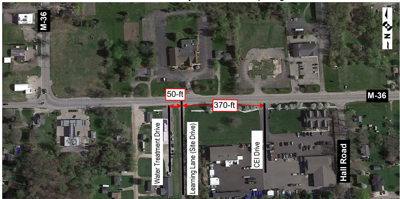
Exhibit 1: Driveway & Intersection Spacing
