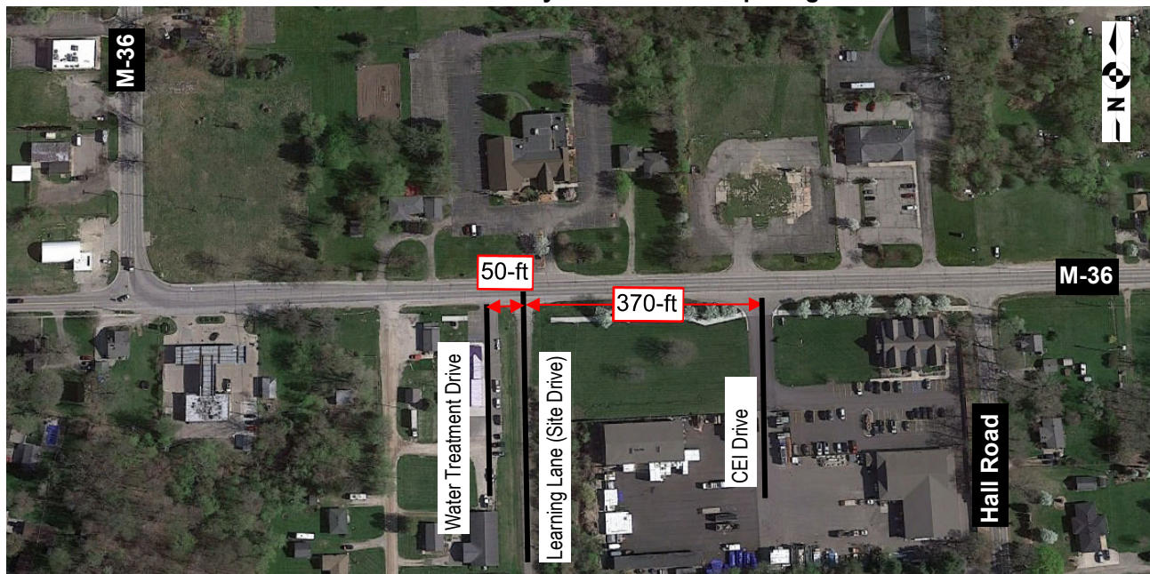
Exhibit 1: Driveway & Intersection Spacing
