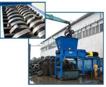
the necessary space for the installation of a shredder.
