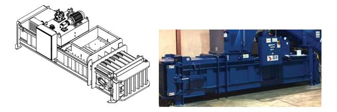
Installation would include the hiring of a construction firm to lift the baler off the shipping flat, move it to its designated place of operation, anchoring it into the concrete, installing any attachments that were removed for shipping, connecting all electrical equipment (disconnect and conduit), and installing hydraulic oil if it was removed for shipping. If a new unit is purchased, final electrical connections and training from the sales staff comes with the purchase.
