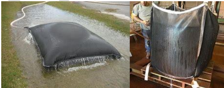
Figure 10. Pumped (left) and gravity-fed (right) geotextile bags.
