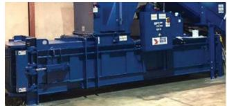
Installation would include the hiring of a construction firm to lift the baler off the shipping flat, move it to its designated place of operation, anchoring it into the concrete, installing any
