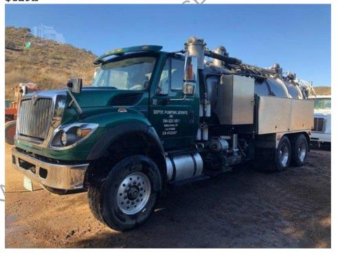
2012 ABCO Industries Mobile Sludge Dewatering Truck- can be used as a traditional pump truck as well. 350 HP Maxxforce 10 motor, 1100 foot pounds of torque 30' long. Dewatering filter rate 50-150 gallons per minute. 10 wheel PDL and differential lock with engine brake. Allison 3500 automatic transmission, air ride seat and backup camera. Custom automated hose reel and electronic control of valves. Hydraulic rear hatch, 800 CFM Wallenstein vacuum pump.
