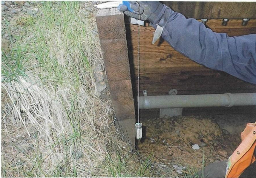
Bridge No. 2320 Br. Name Tong Road Bridge Date 05/19/21 Inspector Bailey / Daugherty Frame 17 NE US Backwall Rotation File P5191028.jpg
