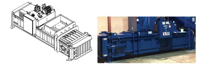
Installation would include the hiring of a construction firm to lift the baler off the shipping flat, move it to its designated place of operation, anchoring it into the concrete, installing any attachments that were removed for shipping, connecting all electrical equipment (disconnect and conduit), and installing hydraulic oil if it was removed for shipping. If a new unit is purchased, final electrical connections and training from the sales staff comes with the purchase.
