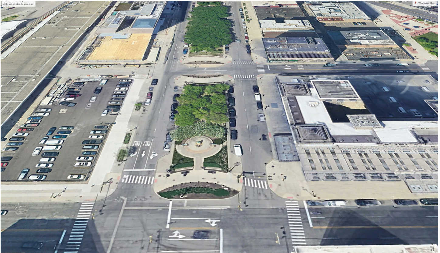
Examples of on-street parking lanes adjacent to medians in Detroit, MI (top: Anthony Wayne Drive, bottom: Washington Boulevard).
