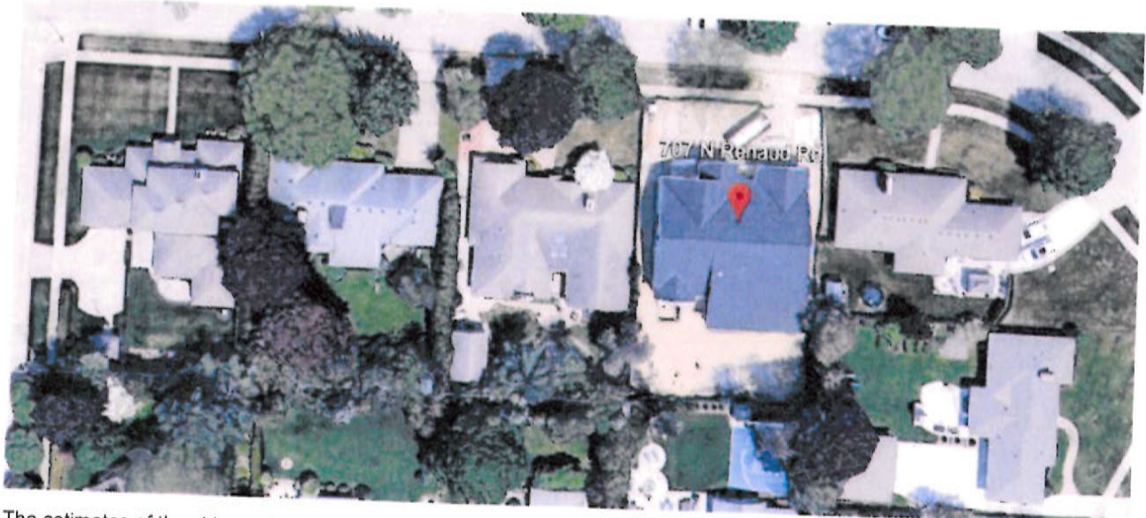
The estimates of the side yard setbacks for houses on this block, based on the Wayne County GIS Parcel Data, include the following, starting at the western corner of the block: House 1 = 10ft / 6ft; House 2 = 4ft / 10ft; House 3 = 4ft / 5ft; House 4
