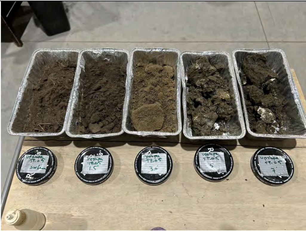
Description: TP-05 Moisture content samples prior to being placed into the drying oven.
