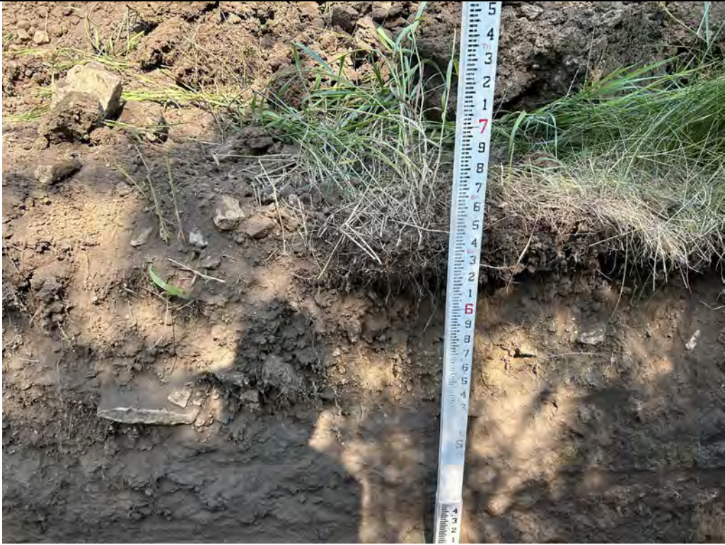
Description: TP-07 Excavated to 6.5 feet.
