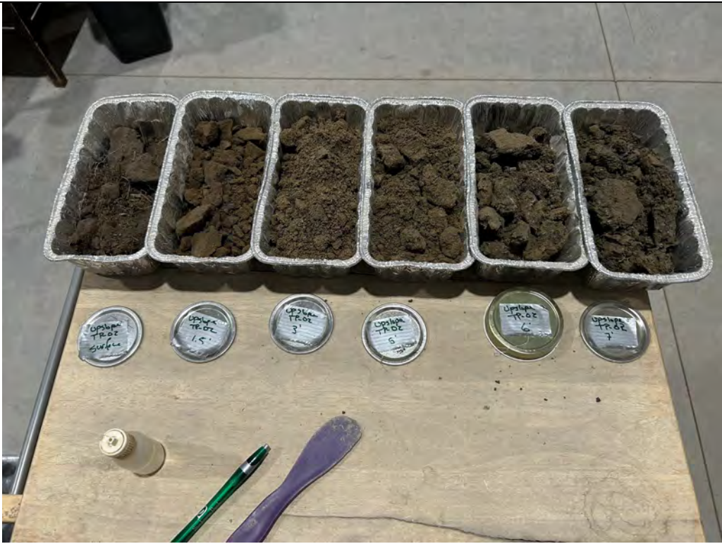
Description: TP-02 Moisture content samples prior to being placed into the drying oven.
