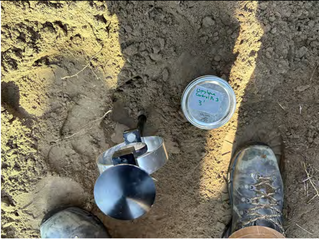
Description: TP-09 Jar sample from 3 feet. Cone penetrometer was pushed 13.75 inches under a 320 psi loading.
