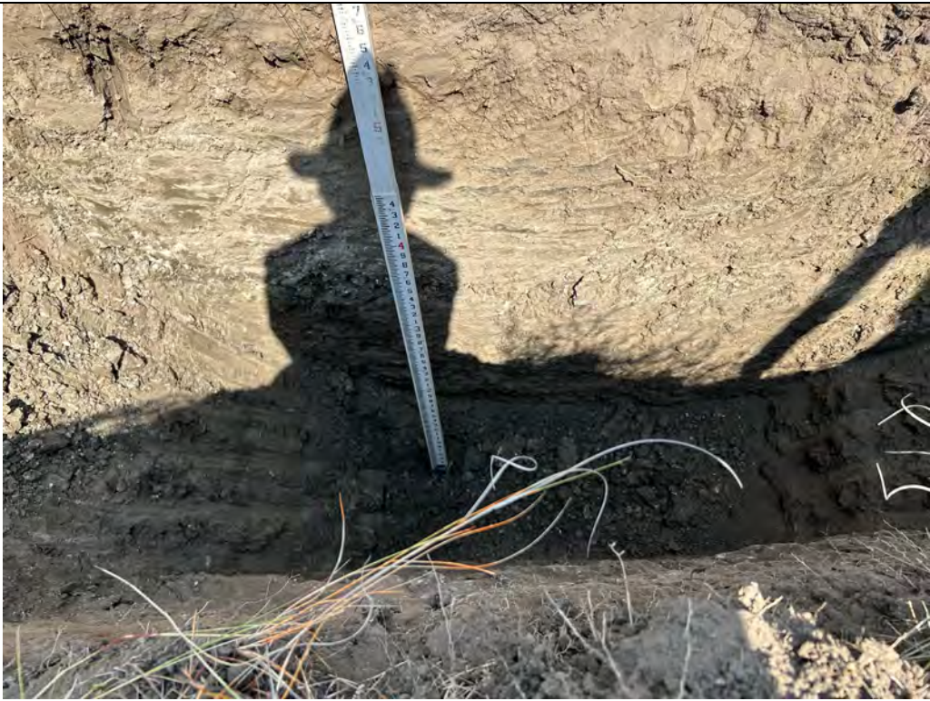
Description: TP-01 Excavated to 6.25 feet.
