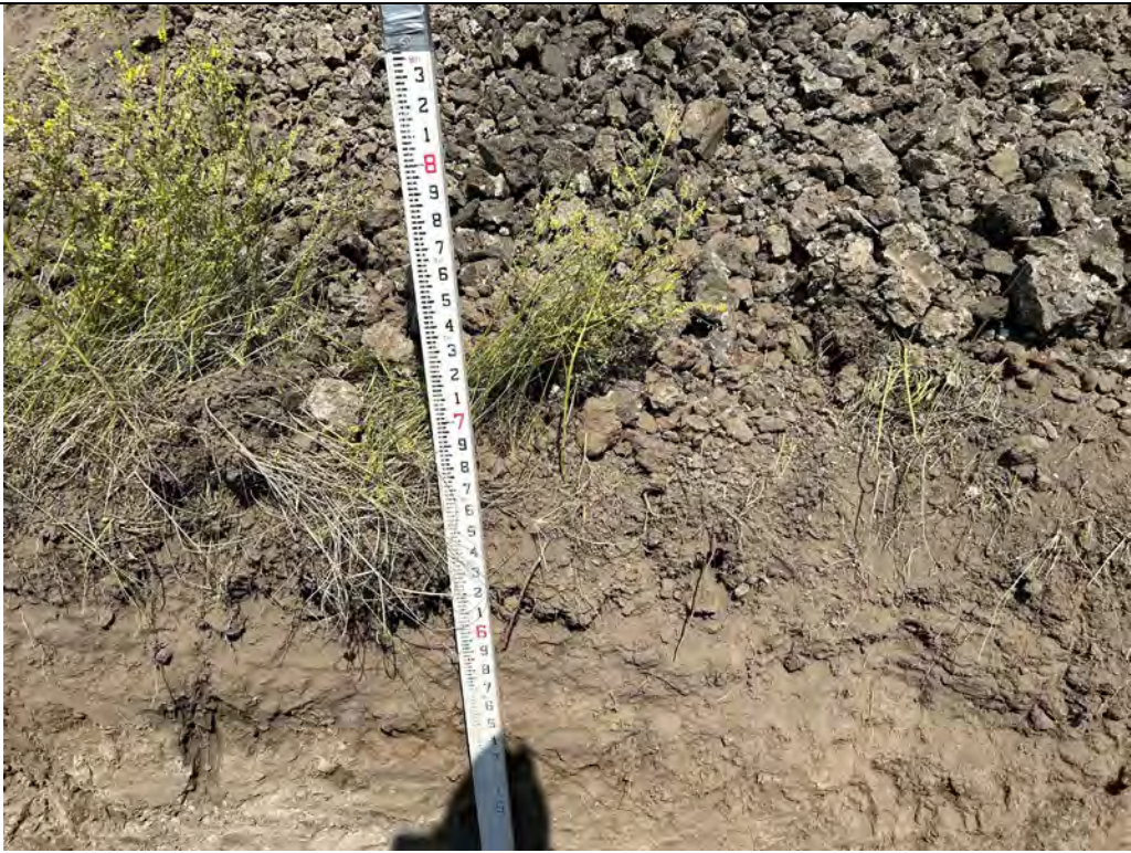
Description: TP-01 Excavated to 6.25 feet.
