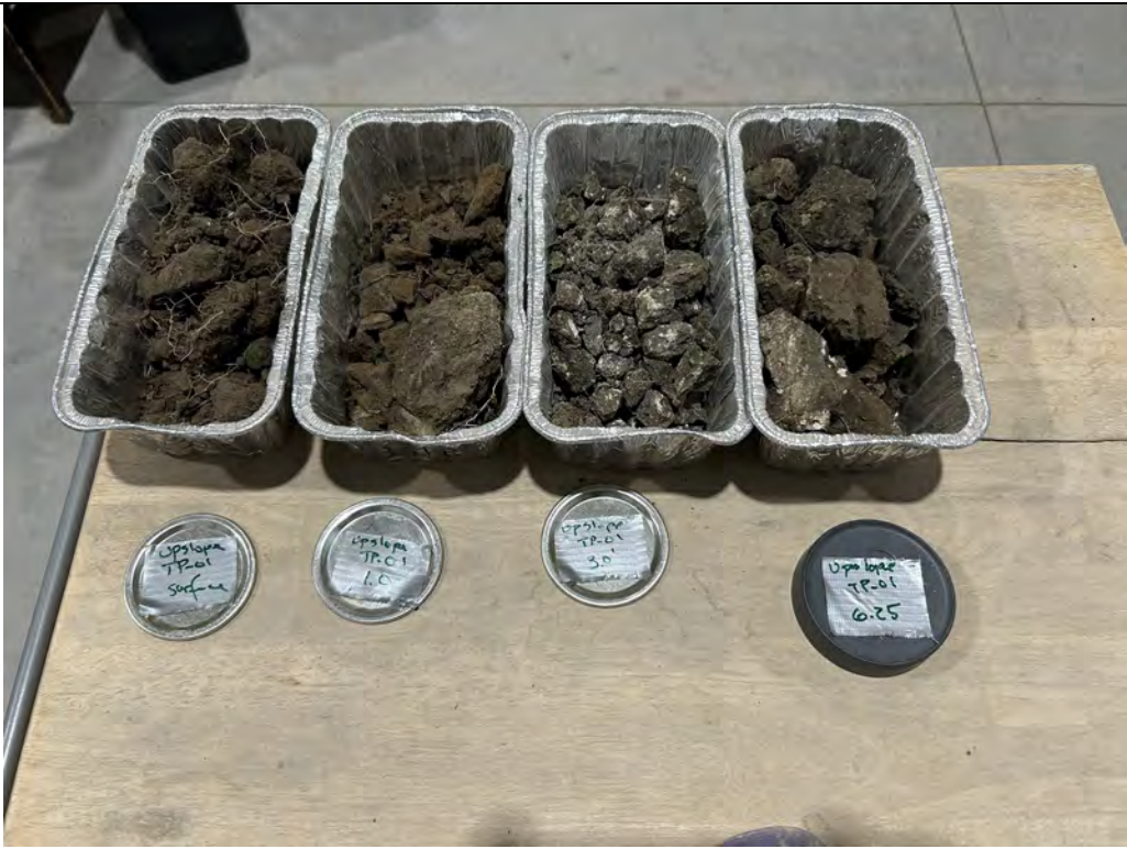
Description: TP-01 Moisture content samples prior to being placed into the drying oven.
