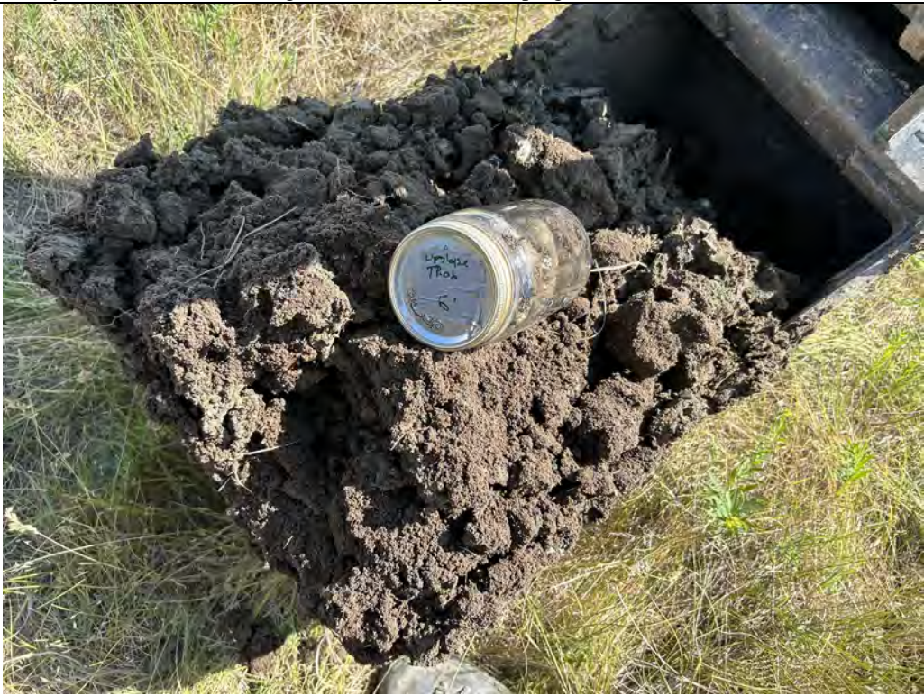
Description: TP-06 Jar sample from 3.75 feet. Cone penetrometer was pushed its full 21 inches under a 280 psi loading. Soil became sticky below 4.5 feet, creating some difficulty in dumping it from the bucket.
