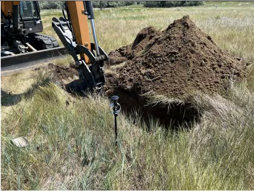
Description: TP-02 Cone penetrometer was pushed 3.25 inches under a 320 psi loading.
