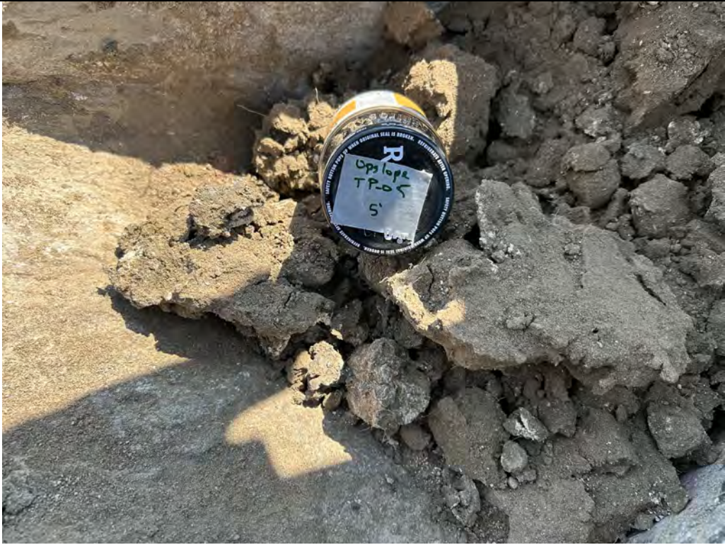
Description: TP-05 Jar sample from 3 feet. Cone penetrometer was pushed 3 inches under a 320 psi loading.
