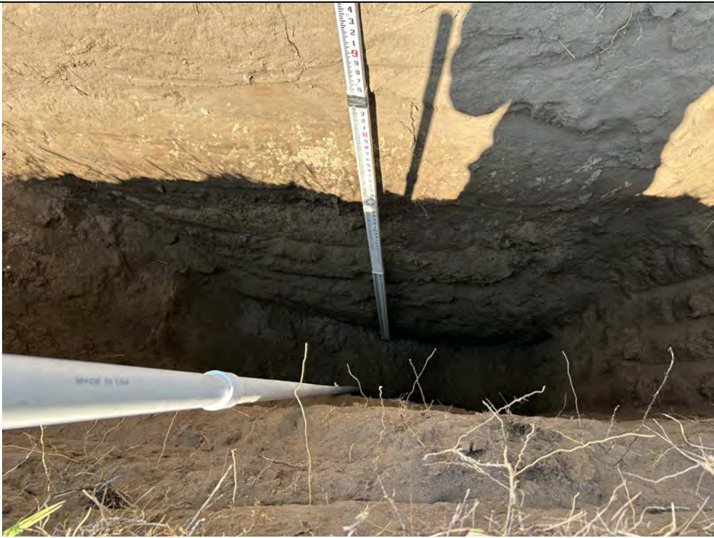
Description: TP-03 Excavated to 8.5 feet.
