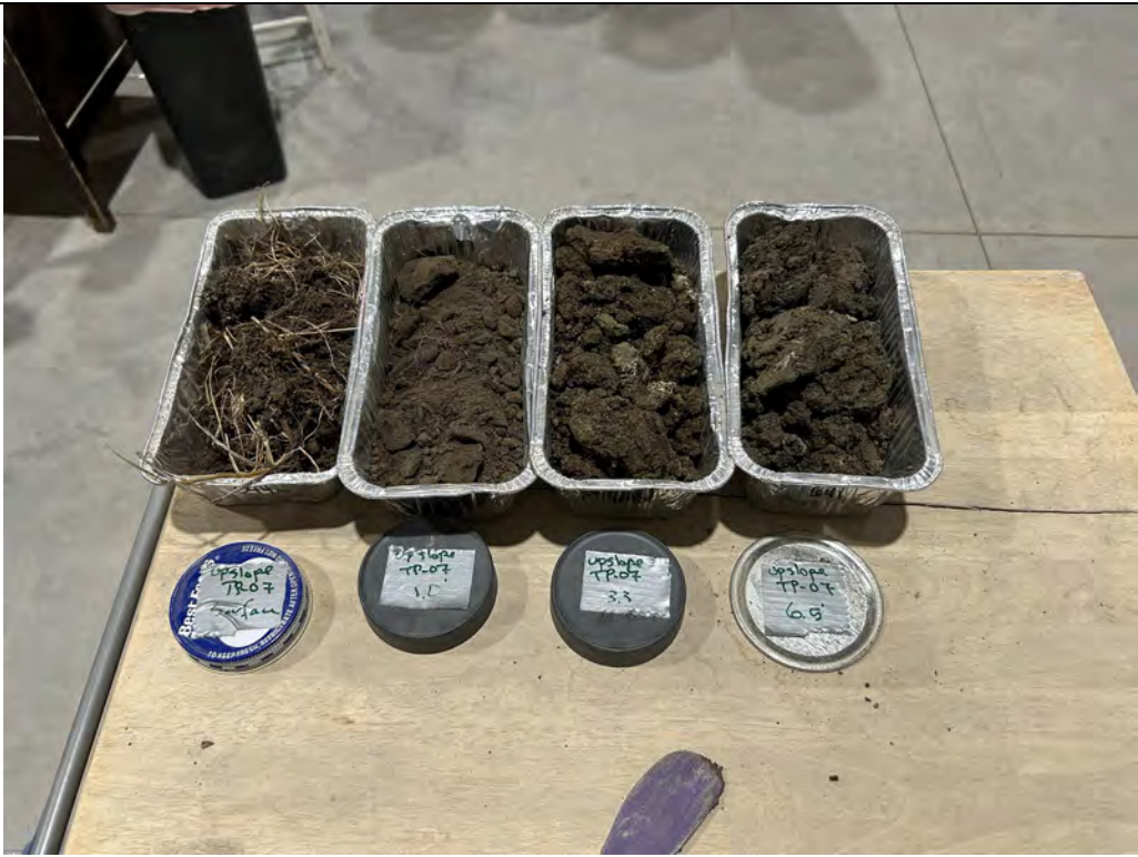
Description: TP-07 Moisture content samples prior to being placed into the drying oven.
