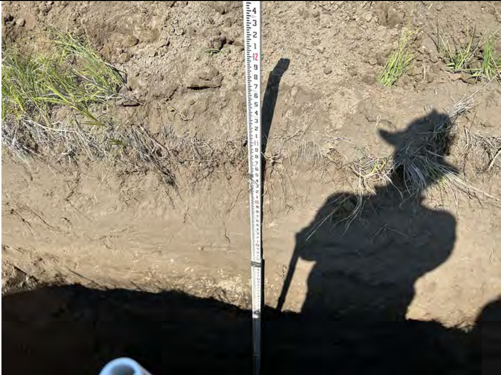
Description: TP-03 Excavated to 8.5 feet.
