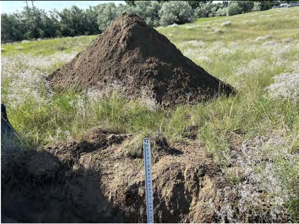
Description: TP-09 Spoils pile from above 11 feet.
