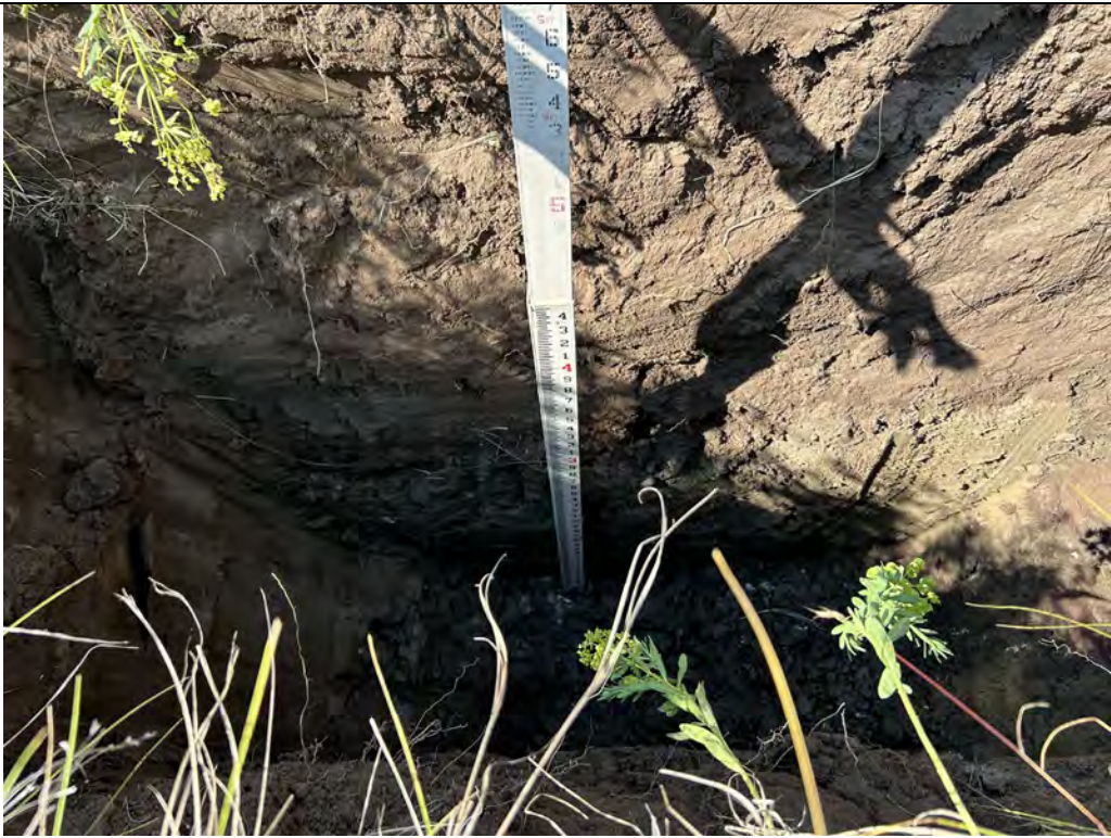
Description: TP-06 Excavated to 6 feet.
