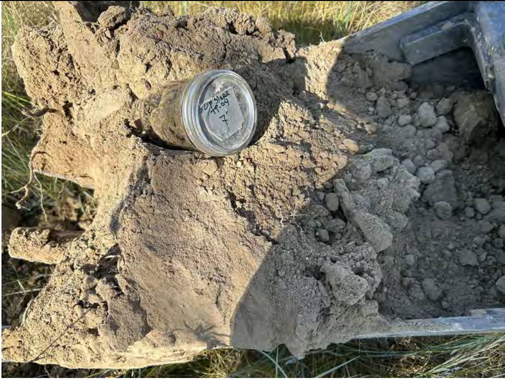
Description: TP-04 Jar sample from 3.4 feet. Cone penetrometer was pushed 12 inches under a 320 psi loading.
