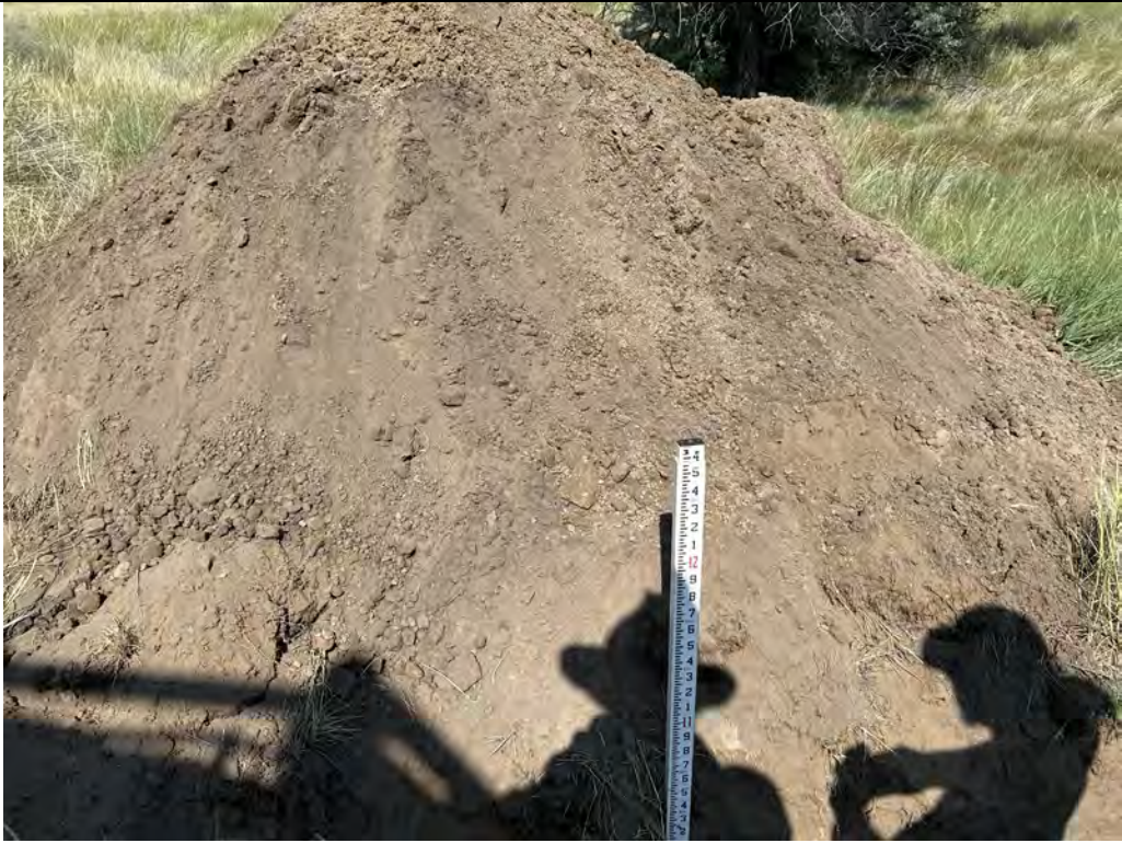
Description: TP-08 Spoils pile from above 10.5 feet.
