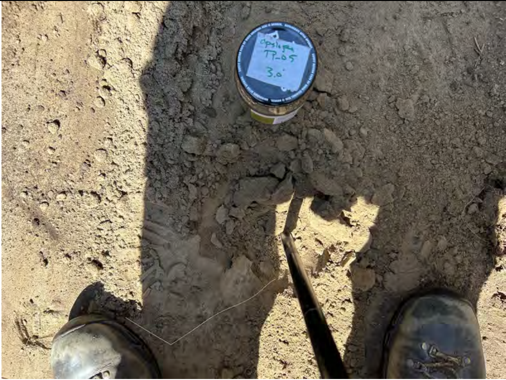
Description: TP-05 Jar sample from 3 feet. Cone penetrometer was pushed 3 inches under a 320 psi loading.
