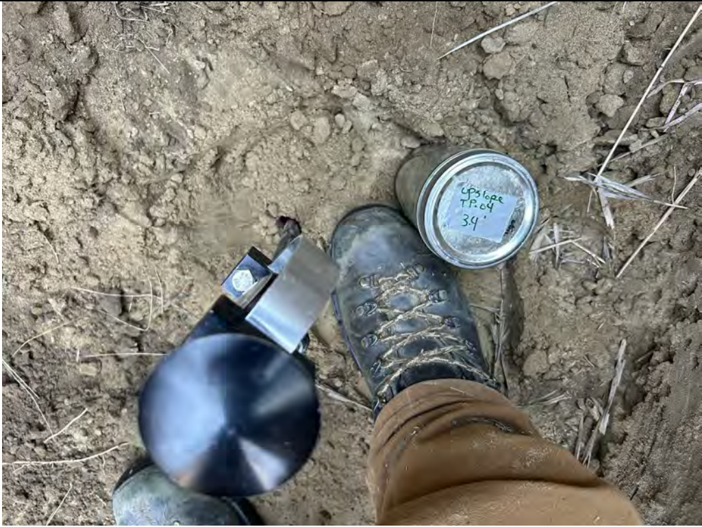
Description: TP-04 Jar sample from 3.4 feet. Cone penetrometer was pushed 12 inches under a 320 psi loading.
