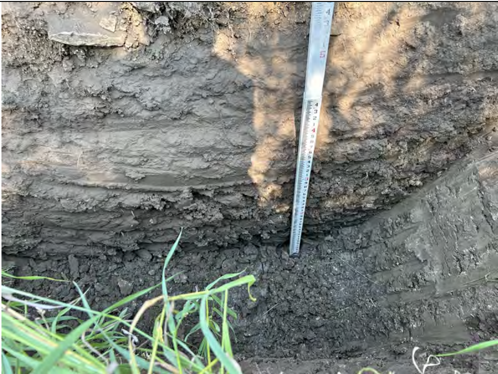
Description: TP-07 Excavated to 6.5 feet.
