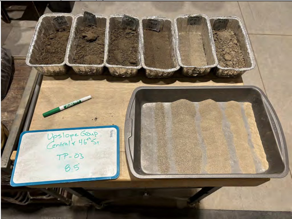
Description: TP-03 Sieved sample of poorly graded sand (SP) from 5.5 feet.
