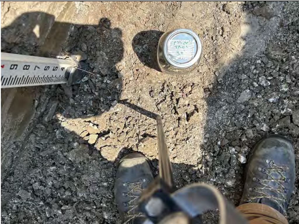
Description: TP-01 Jar sample from 3 feet. Cone penetrometer was pushed 2.5 inches under a 320 psi loading. Jar samples from the ground surface and from 1.5 feet were not photographed.
