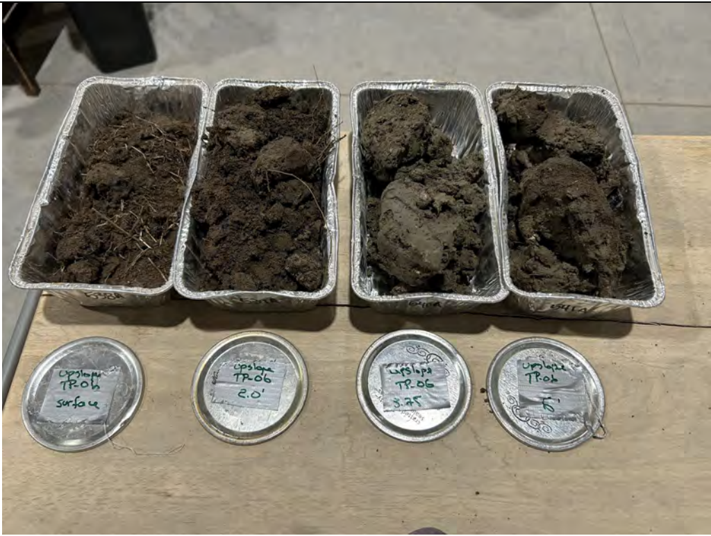
Description: TP-06 Moisture content samples prior to being placed into the drying oven.
