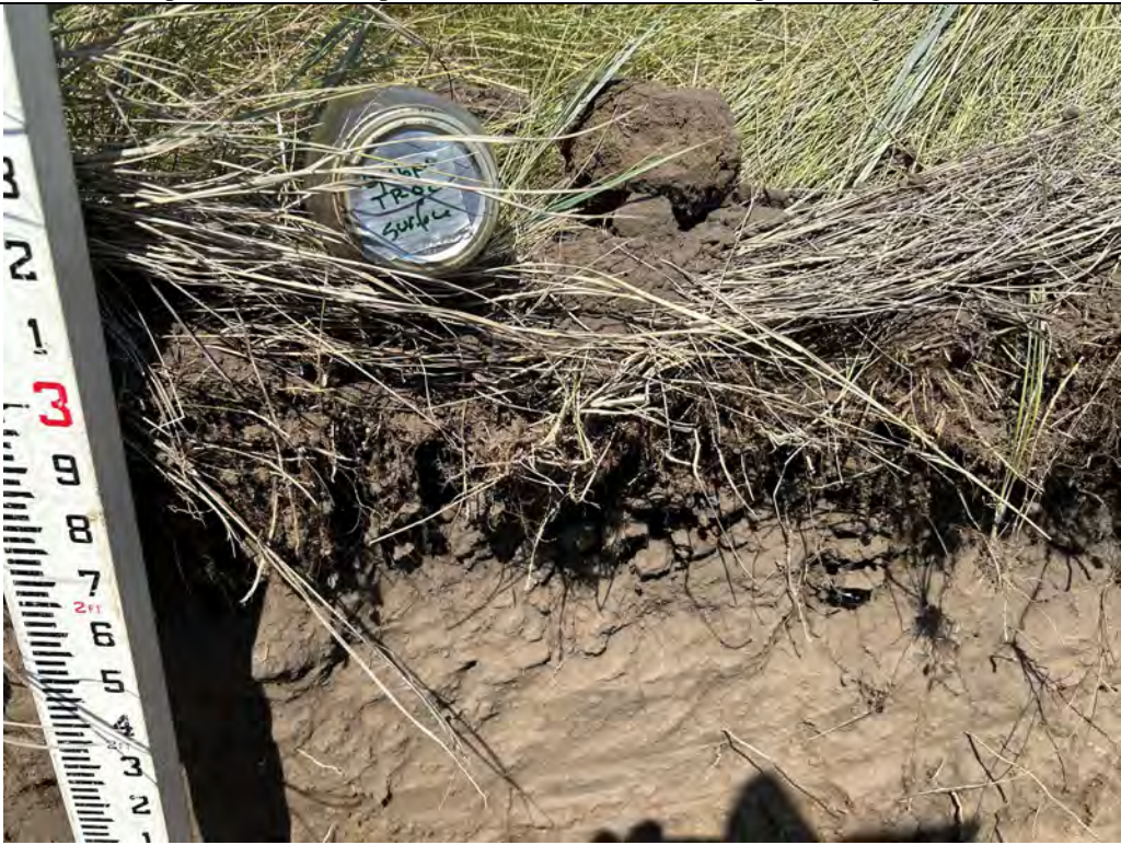
Description: TP-02 Cone penetrometer was pushed 3.25 inches under a 320 psi loading.
