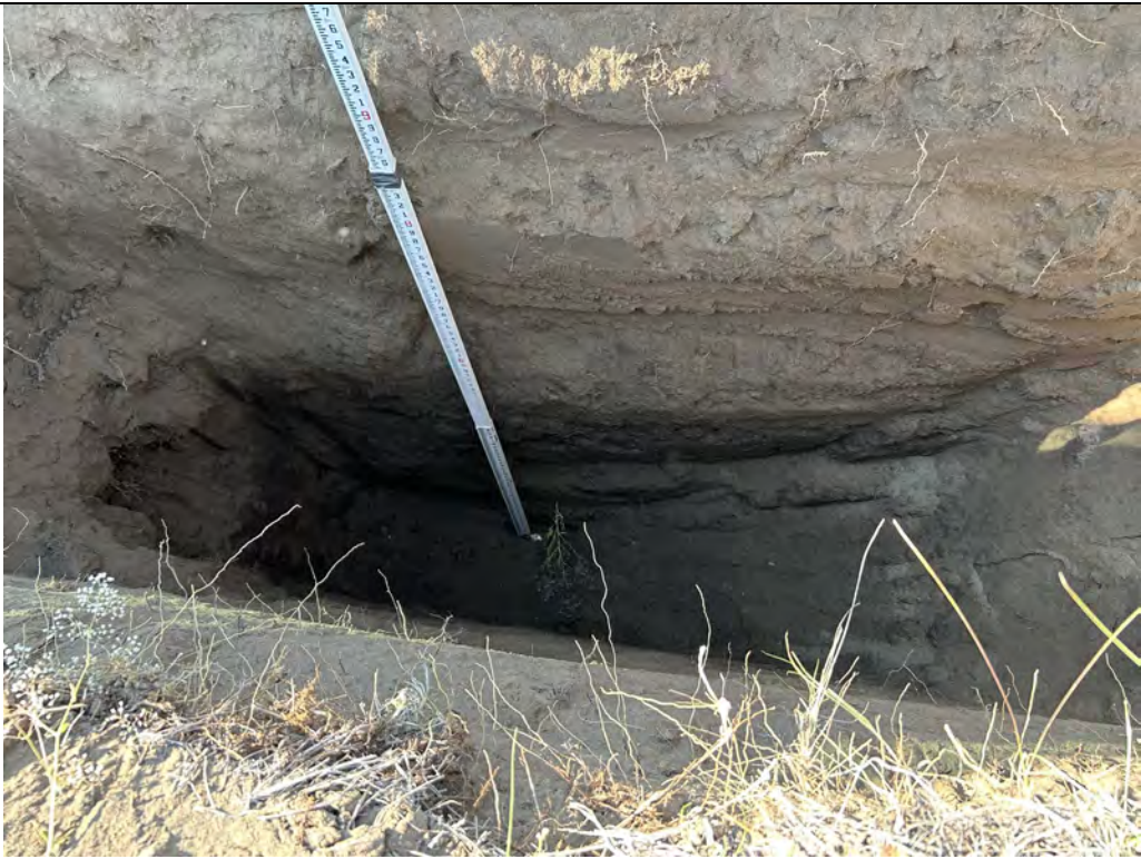
Description: TP-09 Excavated to 11 feet.
