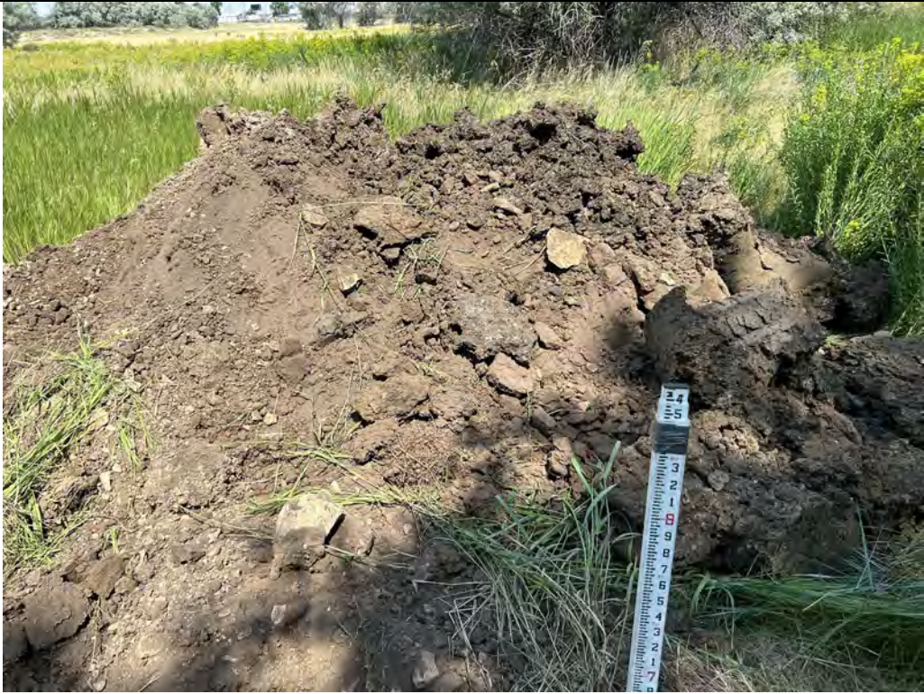
Description: TP-07 Spoils pile from above 6.5 feet.
