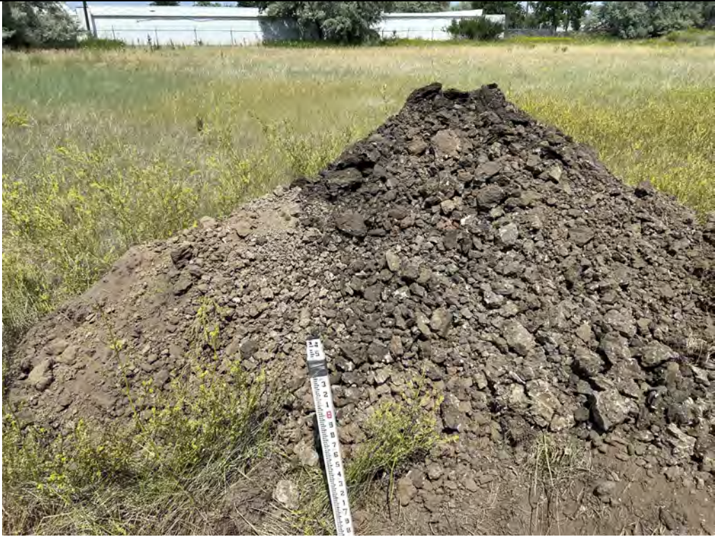
Description: TP-01 Spoils pile from above 6.25 feet.
