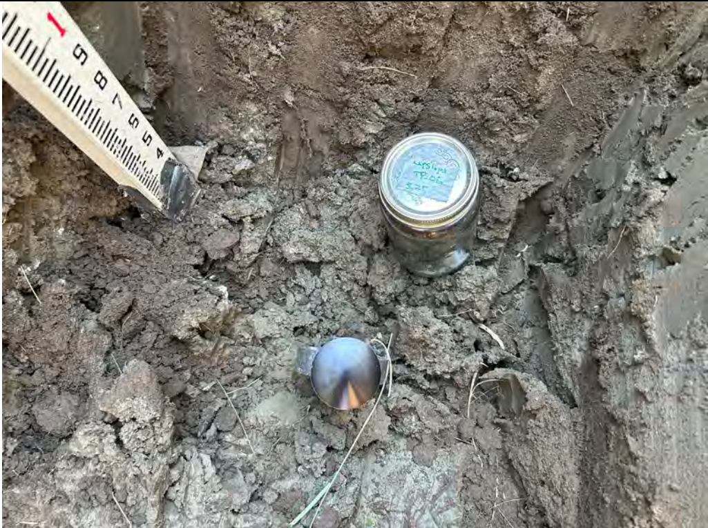
Description: TP-06 Jar sample from 3.75 feet. Cone penetrometer was pushed its full 21 inches under a 280 psi loading. Soil became sticky below 4.5 feet, creating some difficulty in dumping it from the bucket.
