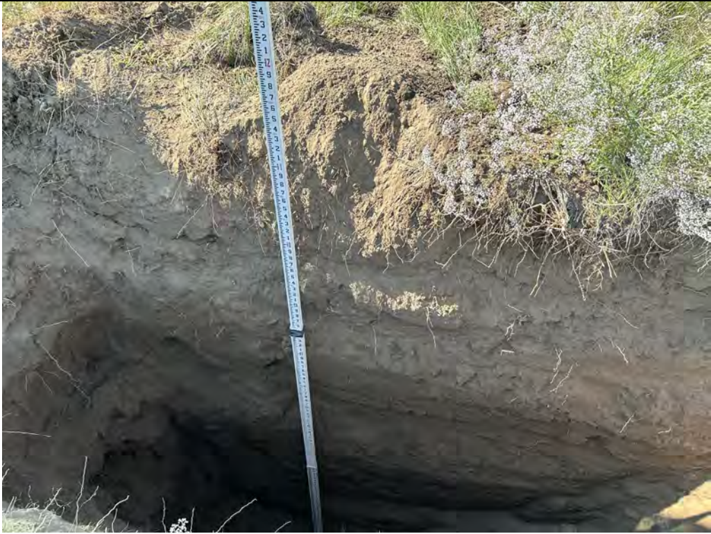
Description: TP-09 Excavated to 11 feet.
