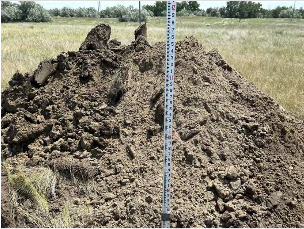
Description: TP-02 Spoils pile from above 7 feet.
