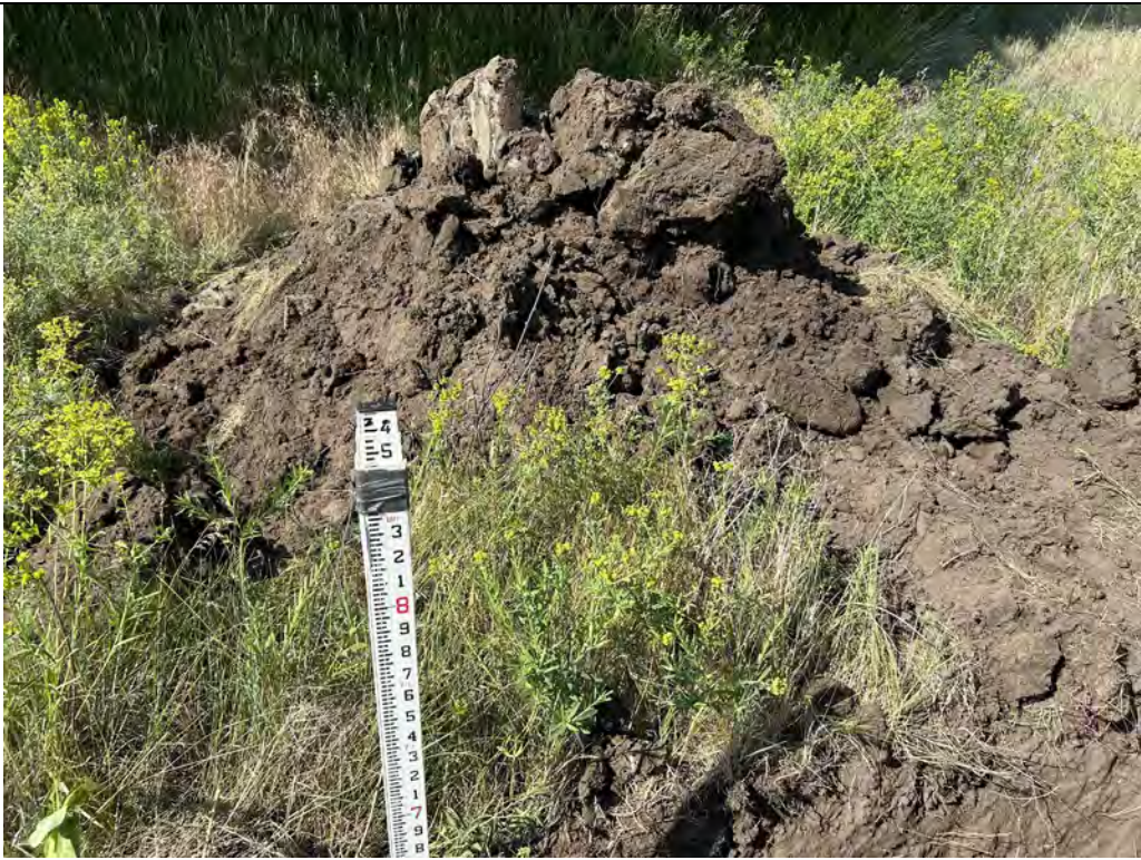
Description: TP-06 Spoils pile from above 6 feet.
