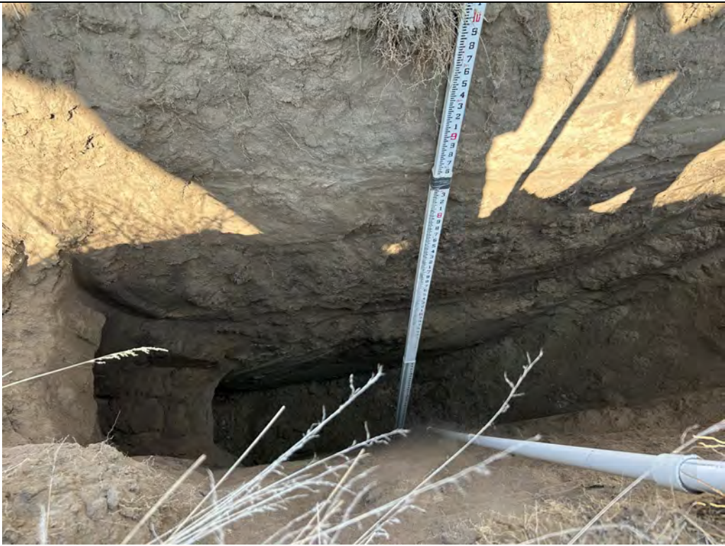
Description: TP-08 Excavated to 10.5 feet.
