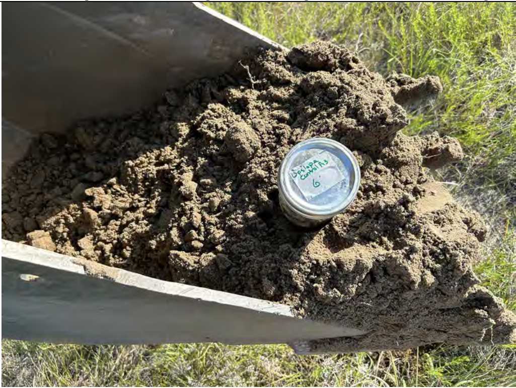
Description: TP-09 Jar sample from 3 feet. Cone penetrometer was pushed 13.75 inches under a 320 psi loading.
