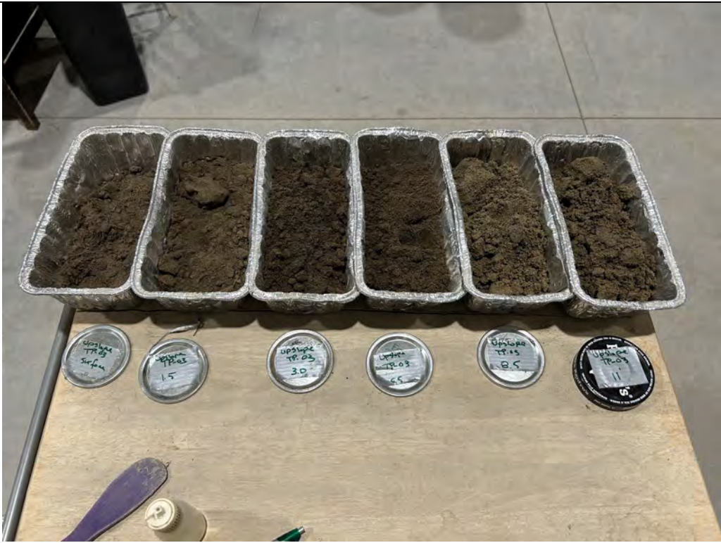
Description: TP-03 Moisture content samples prior to being placed into the drying oven.
