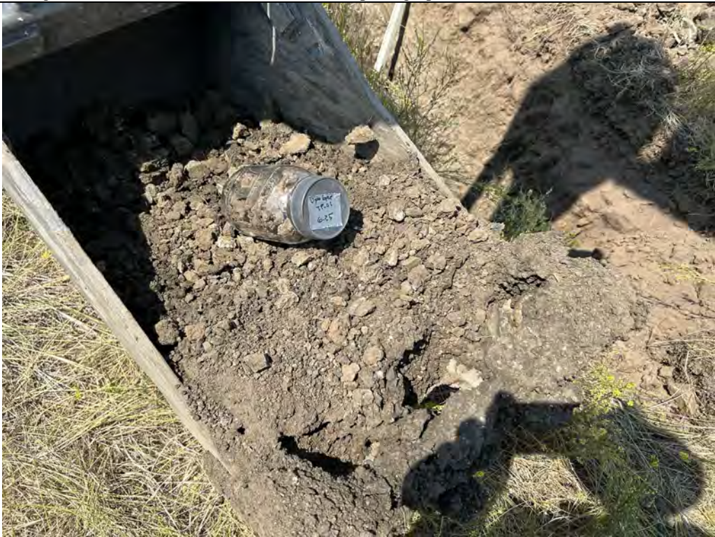
Description: TP-01 Jar sample from 3 feet. Cone penetrometer was pushed 2.5 inches under a 320 psi loading. Jar samples from the ground surface and from 1.5 feet were not photographed.
