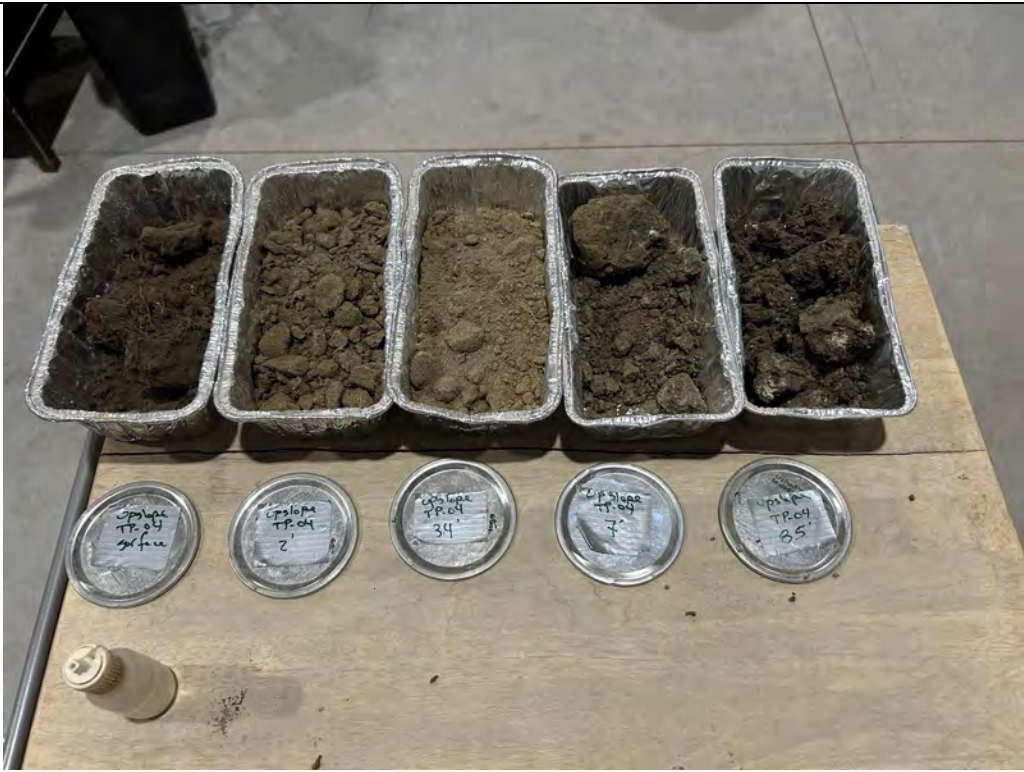
Description: TP-04 Moisture content samples prior to being placed into the drying oven.
