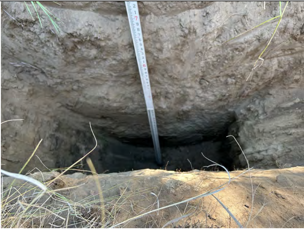
Description: TP-04 Excavated to 8.5 feet.
