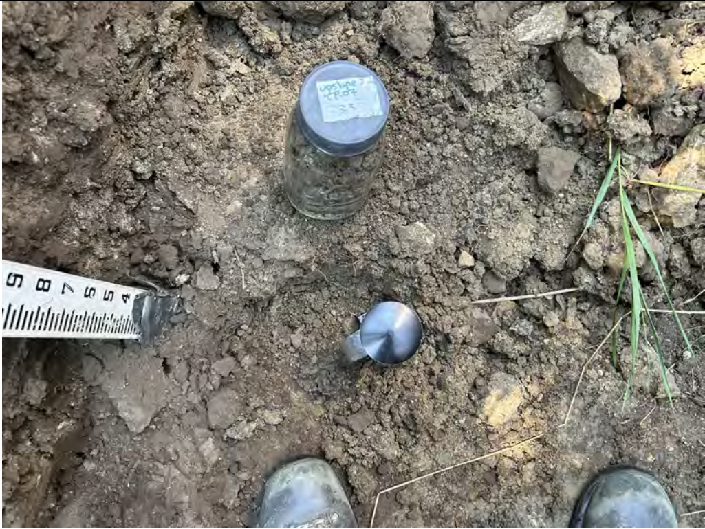
Description: TP-07 Jar sample from 3.3 feet. Cone penetrometer was pushed 16.65 inches under a 320 psi loading.
