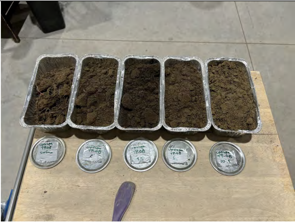
Description: TP-08 Moisture content samples prior to being placed into the drying oven.
