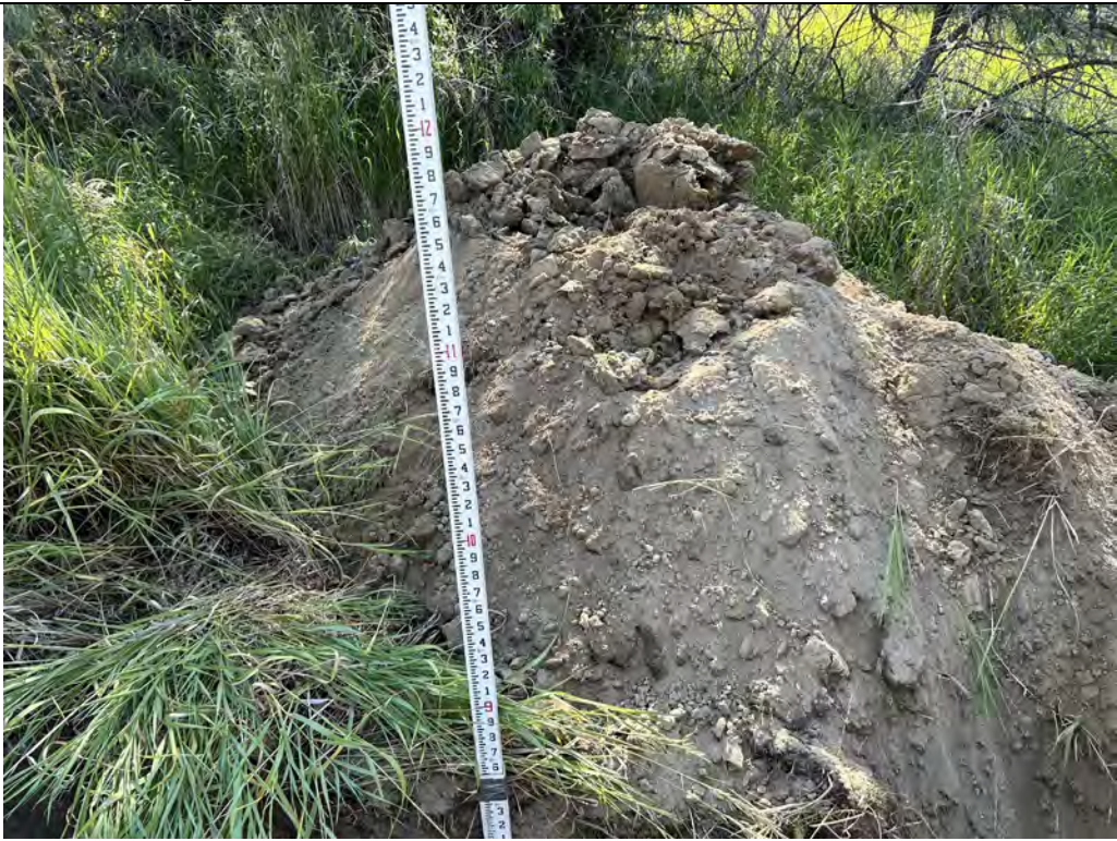
Description: TP-04 Spoils pile from above 8.5 feet.
