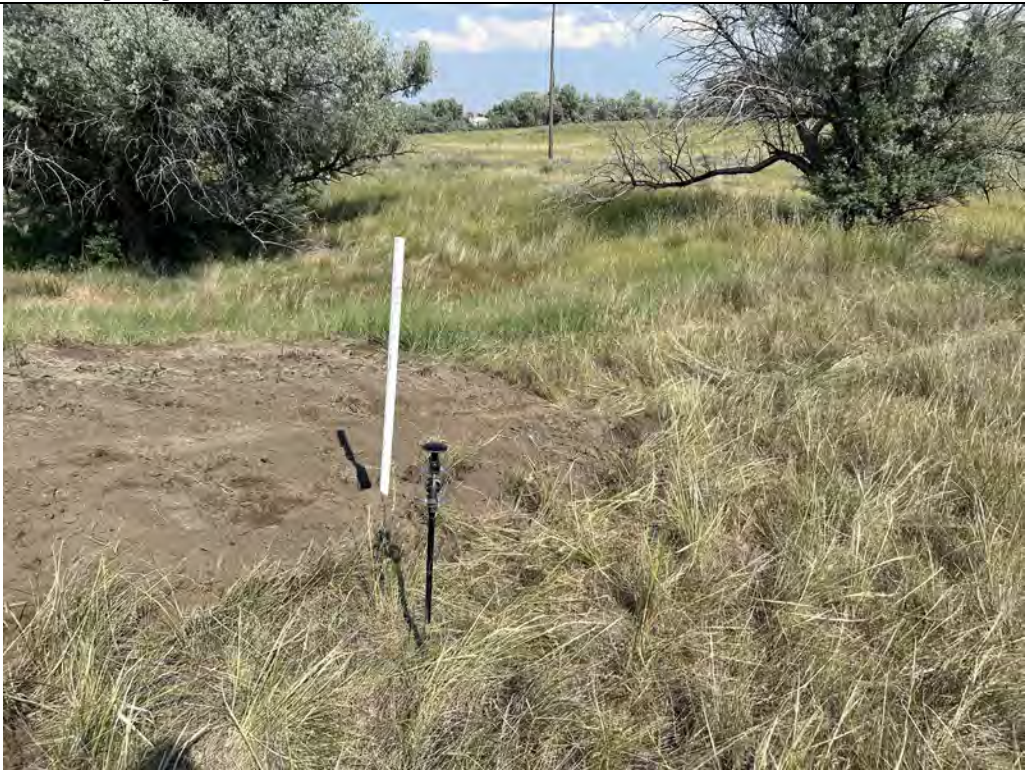
Description: TP-08 Piezometer. Cone penetrometer was pushed 3 inches. View is to the northeast.
