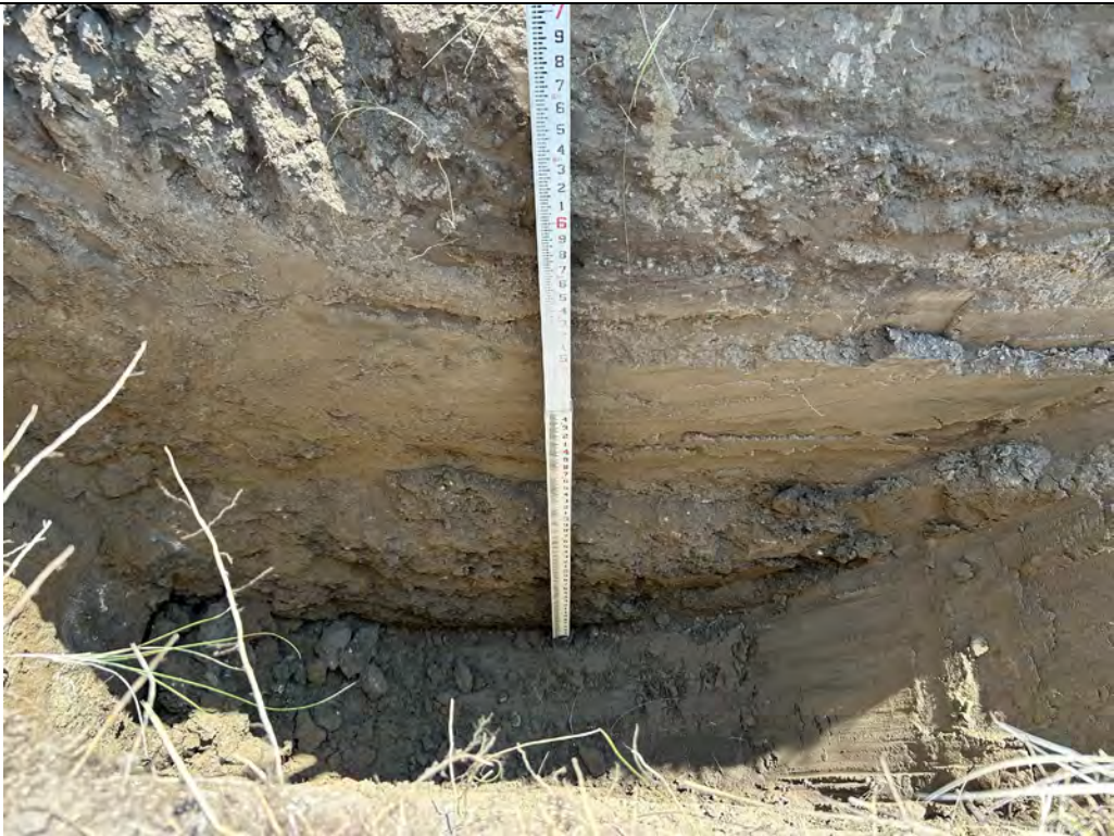
Description: TP-02 Excavated to 7 feet.
