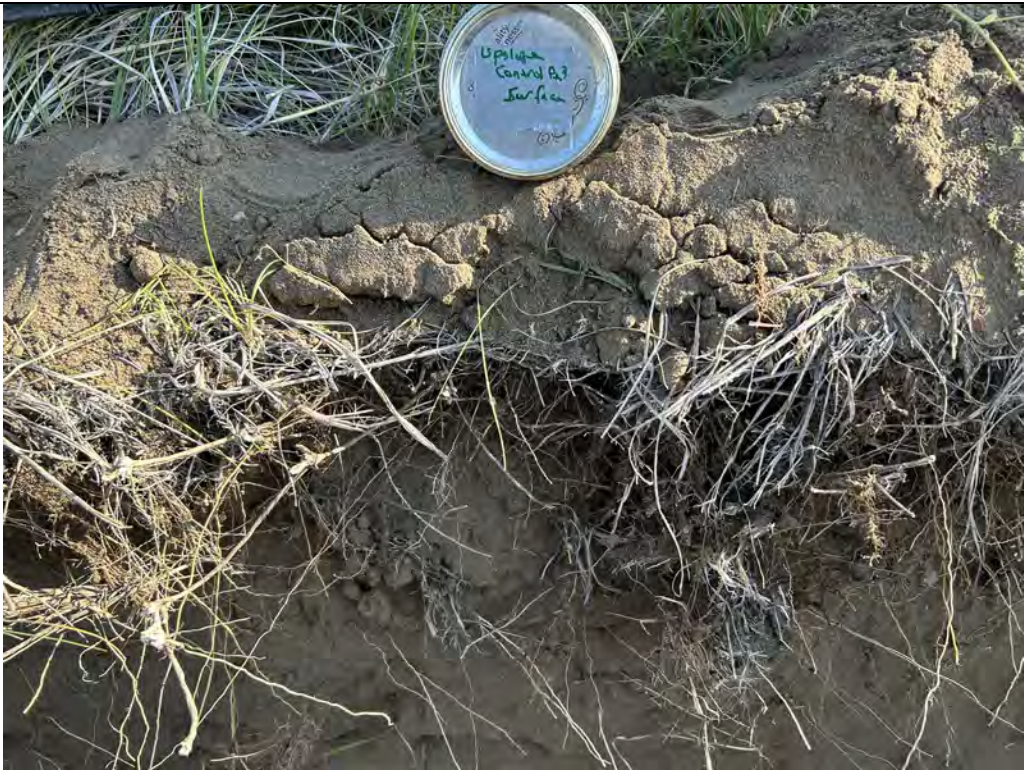
Description: TP-09 Jar sample from the ground surface.
