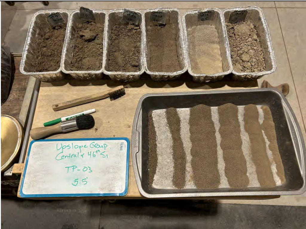
Description: TP-03 Sieved sample of poorly graded sand (SP) from 5.5 feet.
