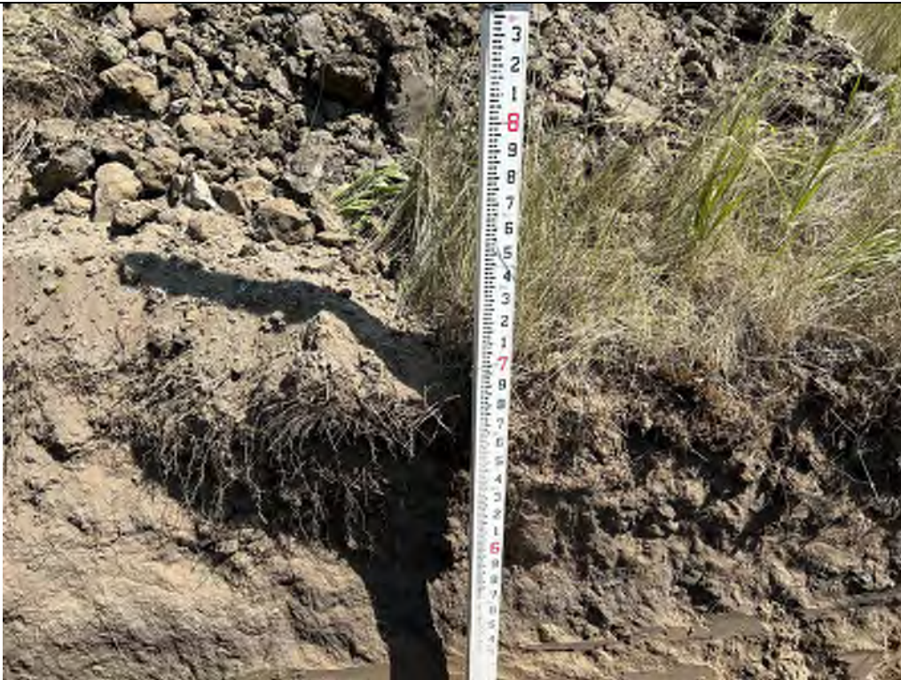
Description: TP-05 Excavated to 7 feet.
