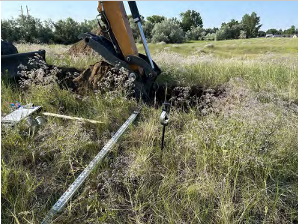
Description: TP-09. Cone penetrometer was pushed 7.25 inches under a 320 psi loading.
