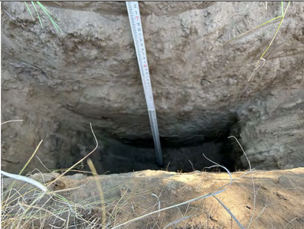
Description: TP-04 Excavated to 8.5 feet.
