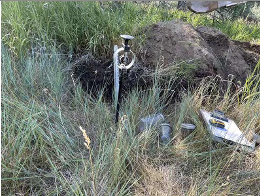
Description: TP-04 Cone penetrometer was pushed 3 inches under a 320 psi loading.
