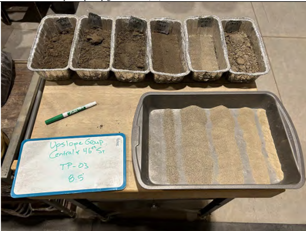
Description: TP-03 Sieved sample of poorly graded sand (SP) from 8.5 feet.
