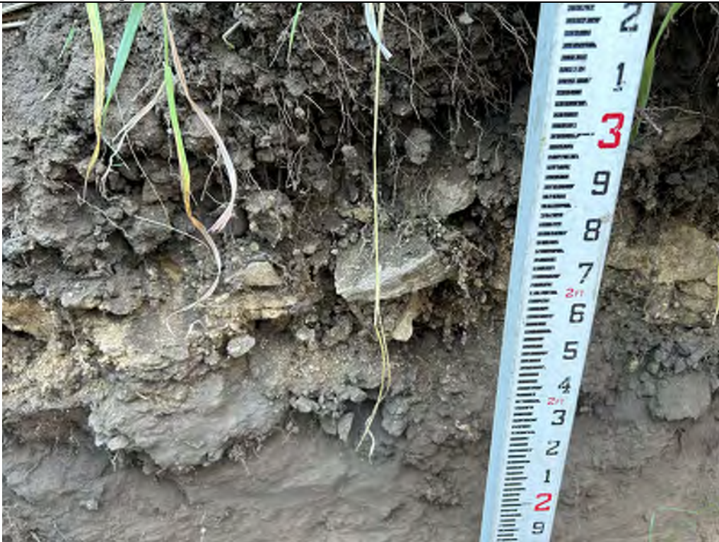
Description: TP-07 Thin rock layer at the 1 foot depth with sand and silt.
