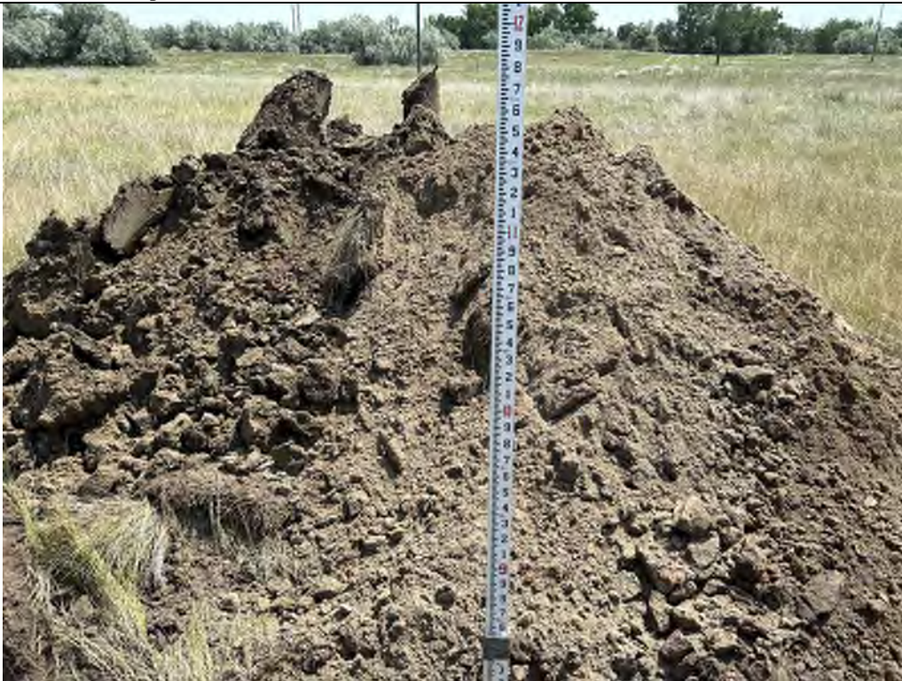
Description: TP-02 Spoils pile from above 7 feet.
