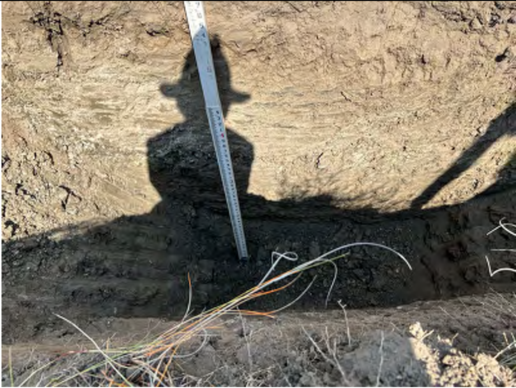
Description: TP-01 Excavated to 6.25 feet.
