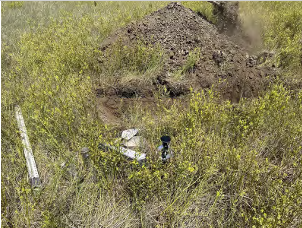
Description: TP-01 Army Corps of Engineers Cone Penetrometer was pushed 7.75 inches under a 320 psi loading.
