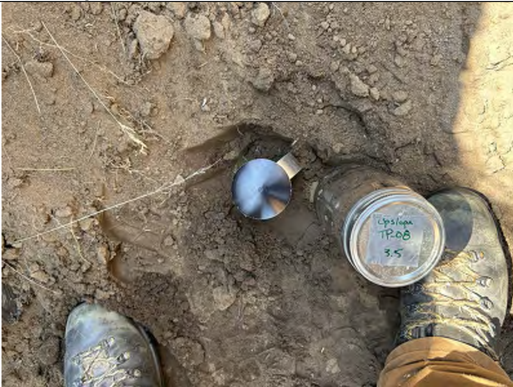
Description: TP-08 Jar sample from 3.5 feet. Cone penetrometer was pushed its full 21 inches under a 260 psi loading.
