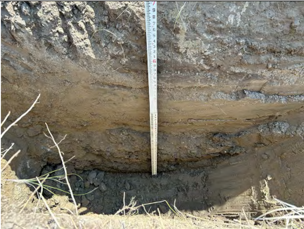
Description: TP-02 Excavated to 7 feet.
