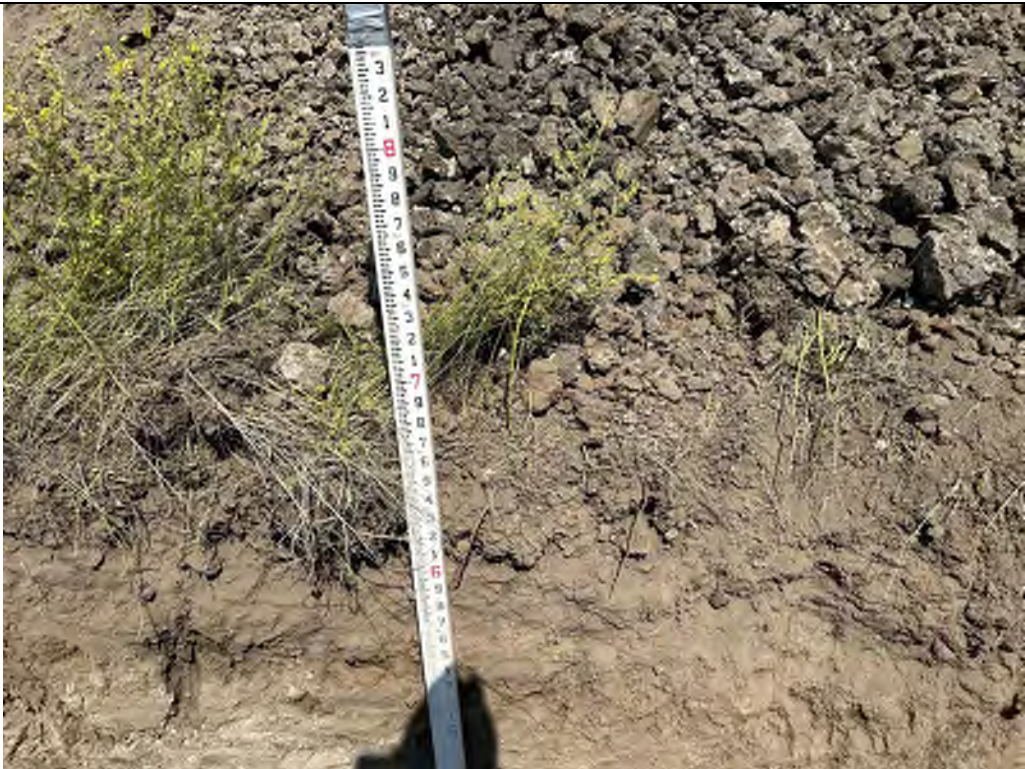
Description: TP-01 Excavated to 6.25 feet.
