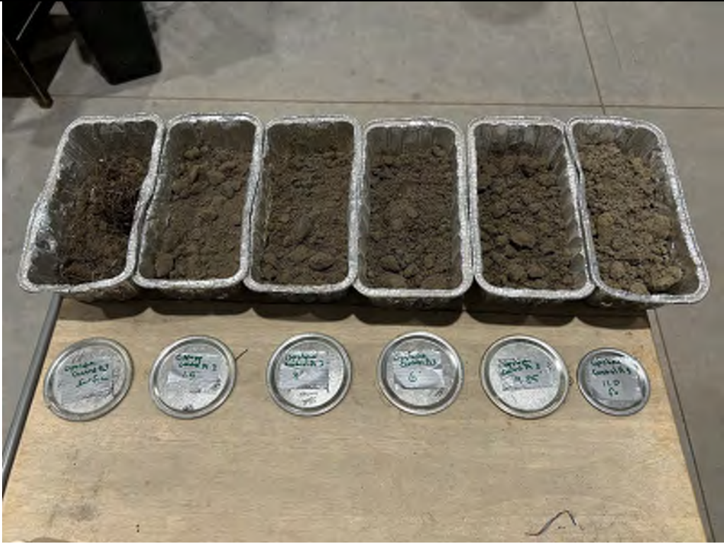
Description: TP-09 [CP-3] Moisture content samples prior to being placed into the drying oven.
