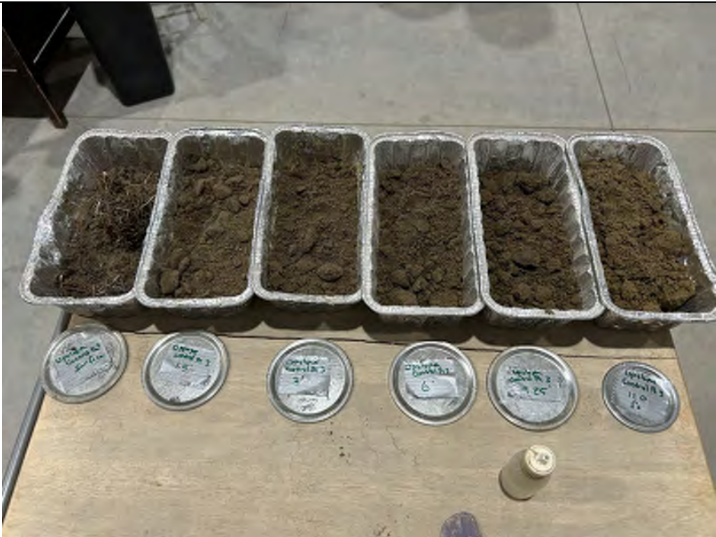
Description: TP-09 [CP-3] Moisture content samples prior to being placed into the drying oven.
