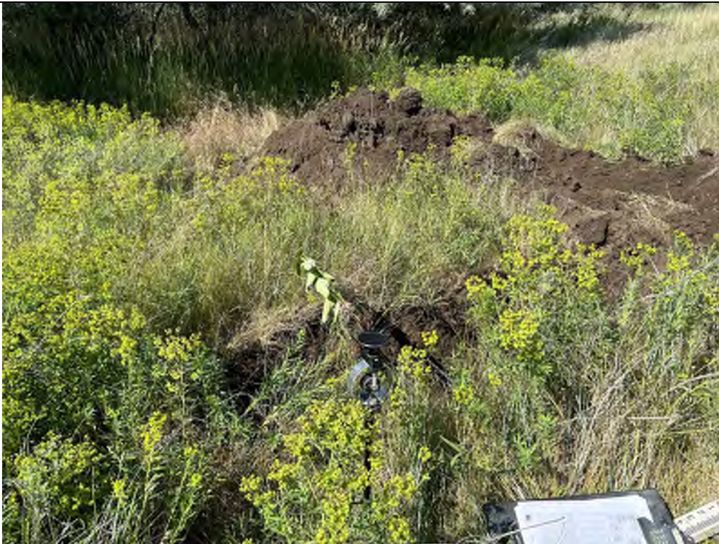
Description: TP-06 Location. View is to the north. Cone penetrometer was pushed 4.25 inches under a 320 psi loading.
