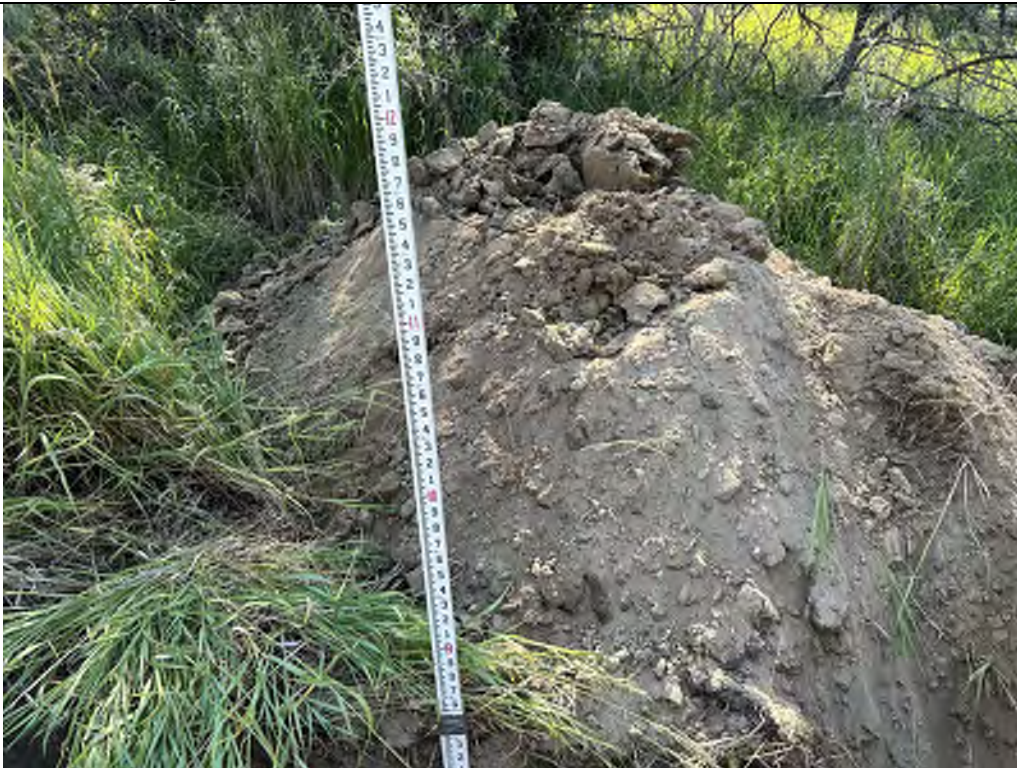
Description: TP-04 Spoils pile from above 8.5 feet.
