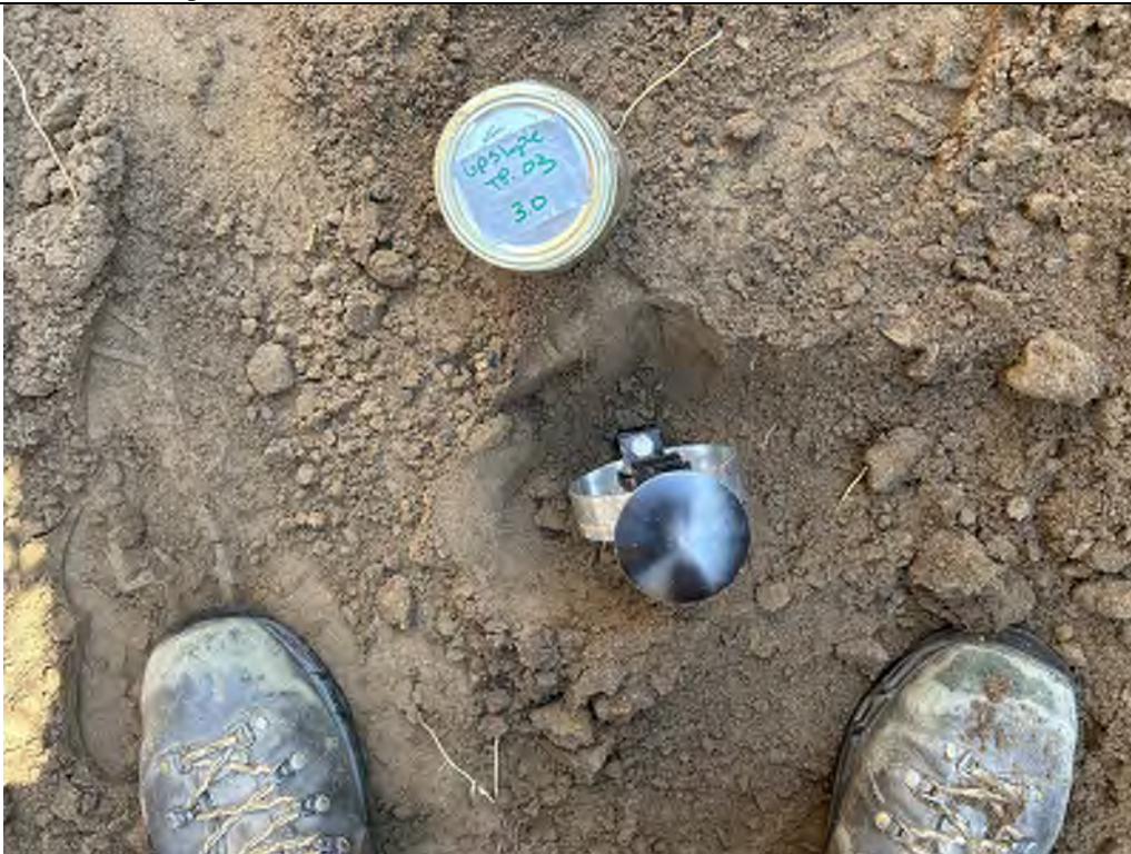
Description: TP-03 Jar sample from 3 feet. Cone penetrometer was pushed its full 21 inches under a 140 psi loading.
