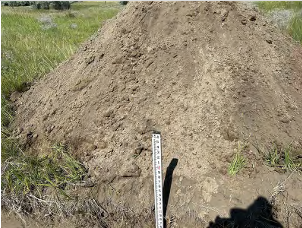
Description: TP-03 Spoils pile from above 11 feet.
