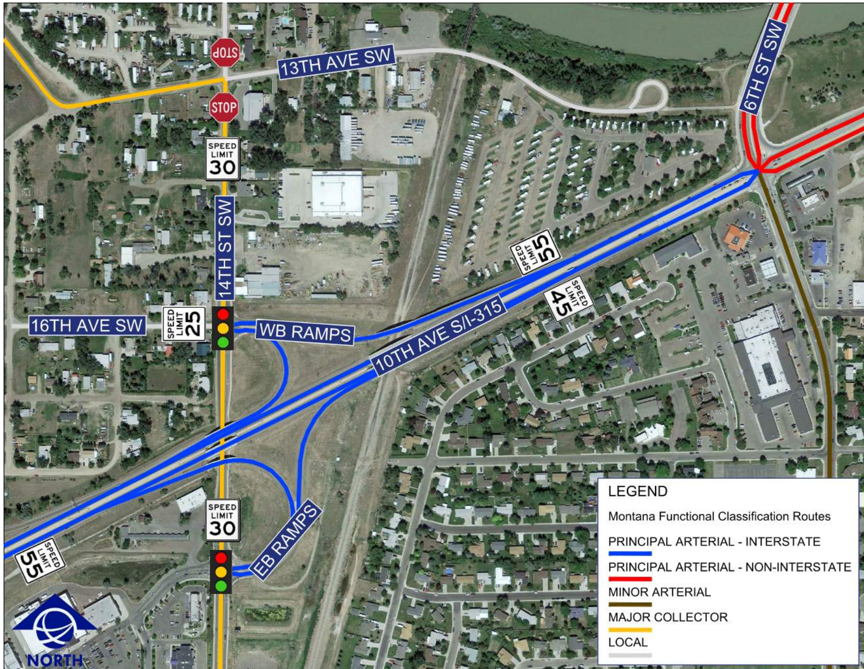
Figure 3: Street & Intersection Characteristics
