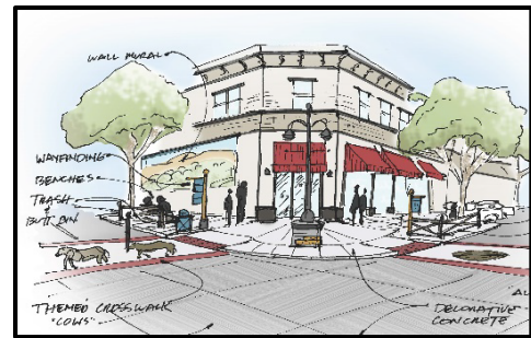
Corner Sidewalk and Crosswalk Design
