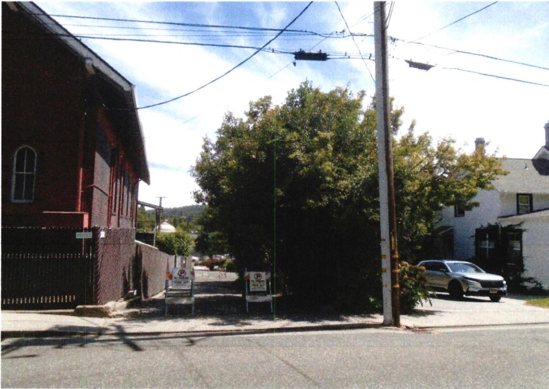
Photo 1 - South School Street. No red/no-parking safety zones flank this constrained commercial driveway. A utility pole occupies a portion of the sidewalk, the Elks fence and Coleman House landscaping substantially obstruct the clear sight distance.
