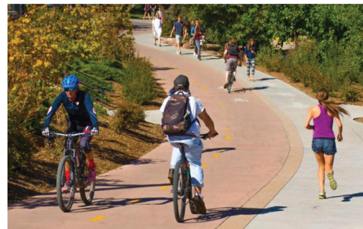
DIFFERENT COLORED CYCLIST AND PEDESTRIAN PAVINGS DESIGNATE USAGE TYPE. BOULDER CREEK BIKE TRAIL. BOULDER, CO.
