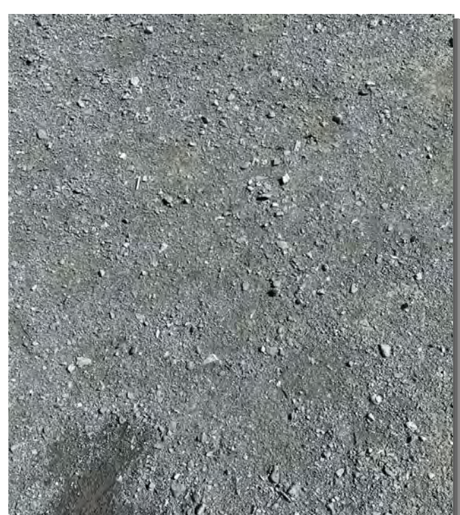
TRAIL SURFACE (BLUE MINER'S GRAVEL)
