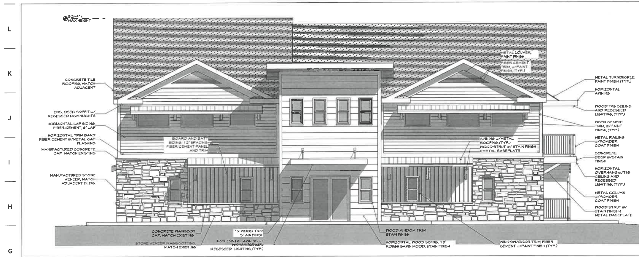
G15 EAST ELEVATION - NEW BUILDING 1/4" = 1'-0"
