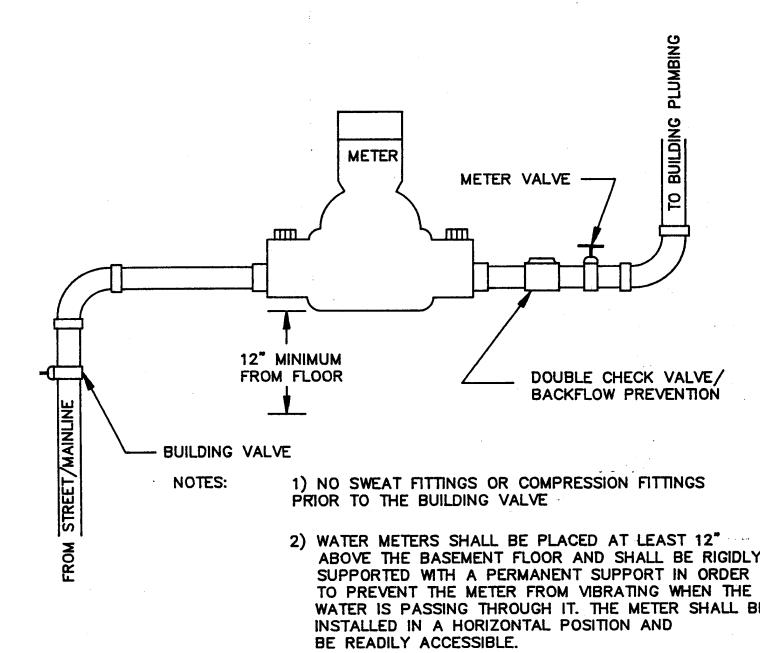
TYPICAL WATER METER INSTALLATION
