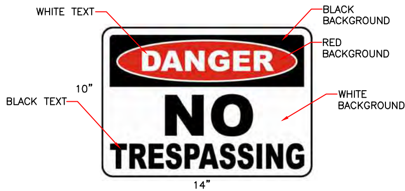
DANGER NO TRESPASSING SIGN WHITE/BLACK BACKGROUND, BLACK/WHITE LETTERING MOUNTING LOCATION: GATE & BASE OF TOWER QUANTITY: 1
