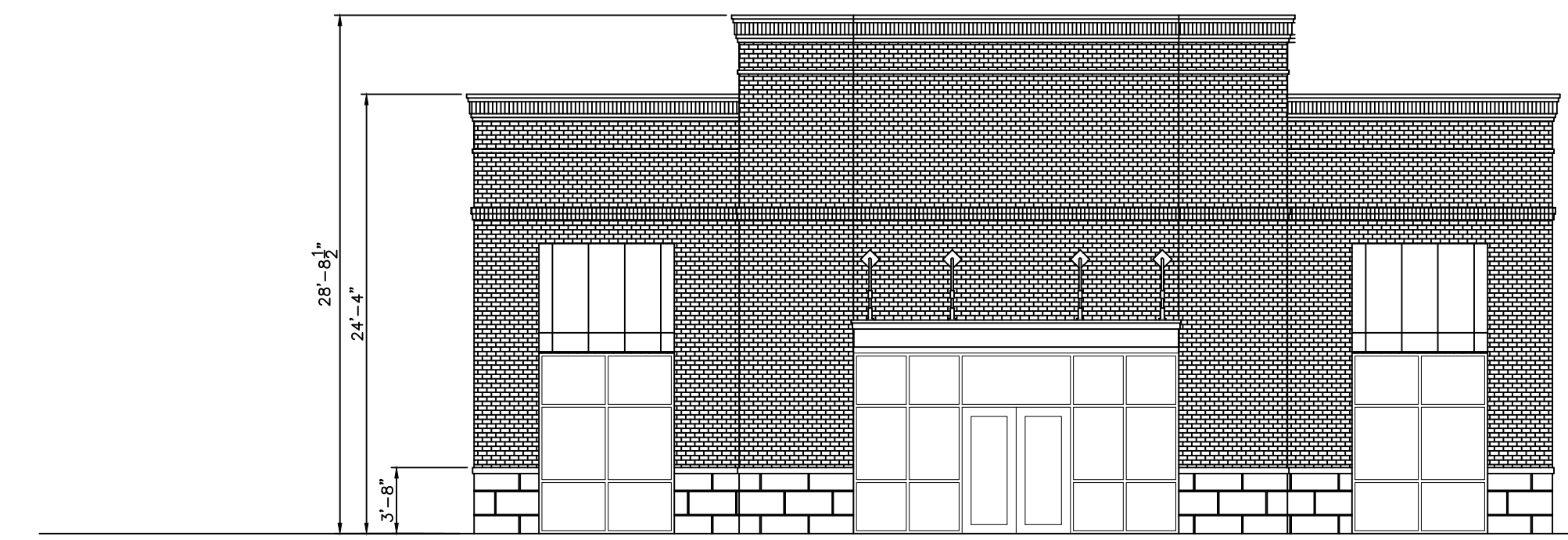
1 SOUTH ELEVATION A1.0 SCALE: 1/8"=1'-0"
