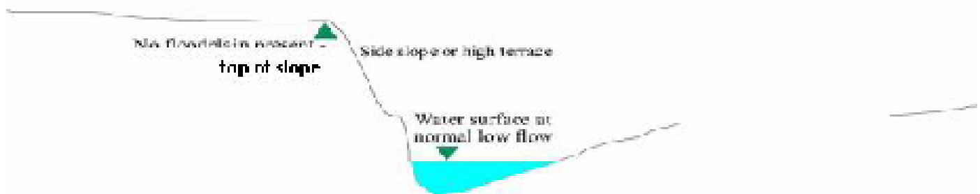
Figure 10.3. Top of slope typical of streams that run adjacent to steep slopes or high terraces on one side of the valley but have adequate floodplain on the opposite side of the valley.
