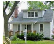
Shed dormers have a single, inclined roof.
