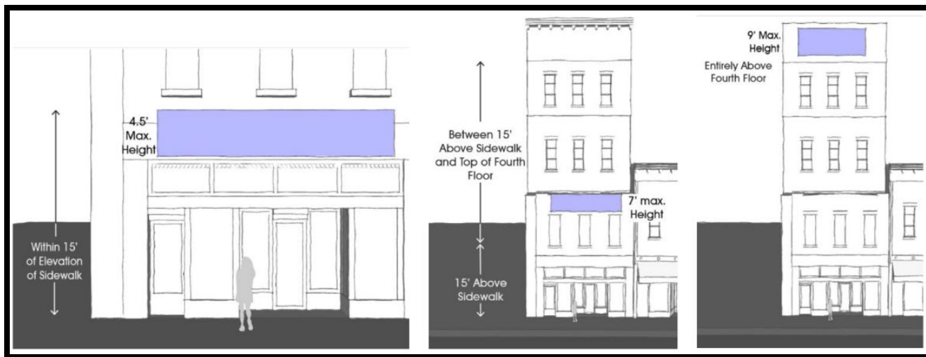
Figure (B)(1) Applied or Painted Wall Signs
