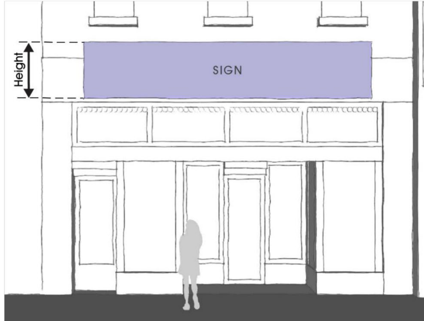
Figure (F)(4)(b) Sign Height (Building-Mounted Signs)
