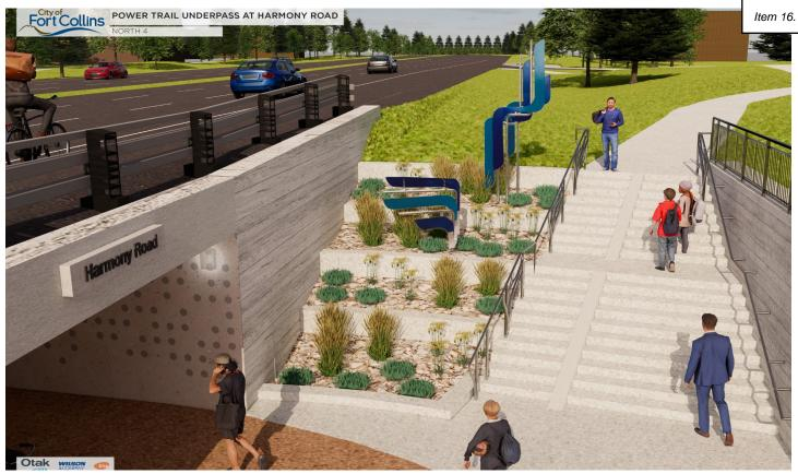
East elevation rendering of *Motus Aquae (Movement of Water)* by artist Todd Kundla . 8' x 12' x 12' with 3" x 6" steel rectangular tubing, oxidized finish, 1/2" thick polycarbonate colored panels (7x stronger than glass)
