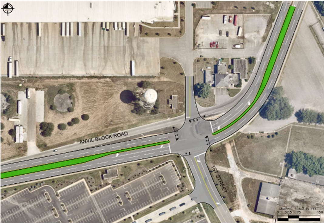
Figure 2: Alternative 2 - Traffic Signal with Realignment
