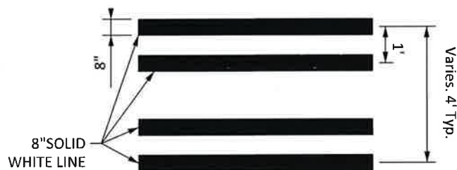
ENTRY BUFFER STRIPING DETAIL N.T.S.
