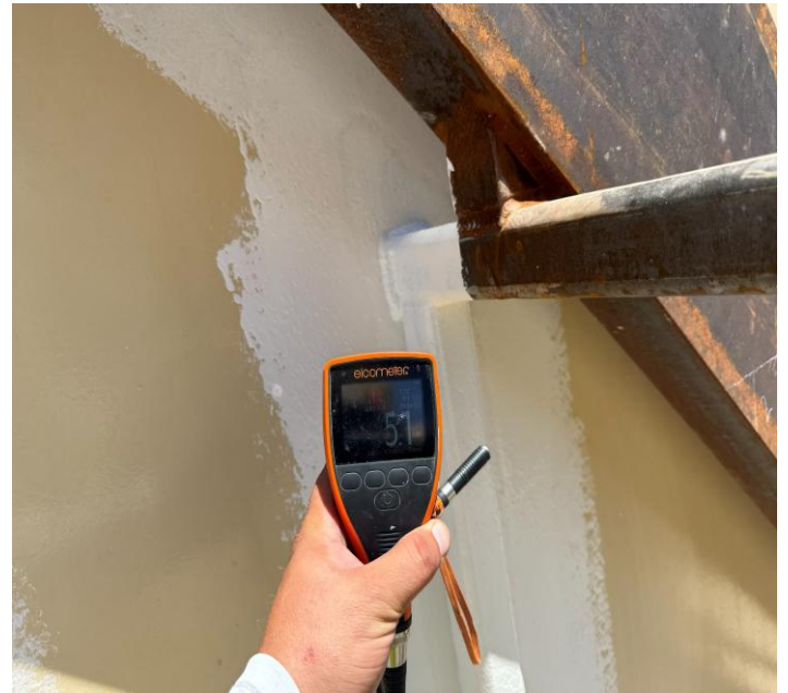
Lower sections of bare metal spot primed areas contained acceptable mil ranges.
