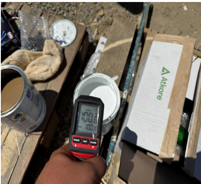
Coating material temperature at 100°F
