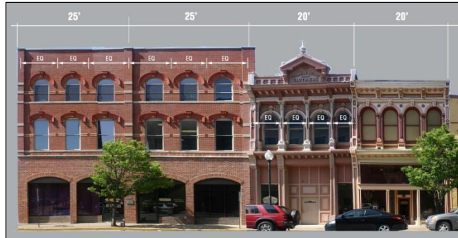
Figure 7-3 6.6 Illustration showing building articulation requirement
