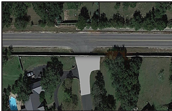
Figure 22 – Partial Hammerhead Turnaround
