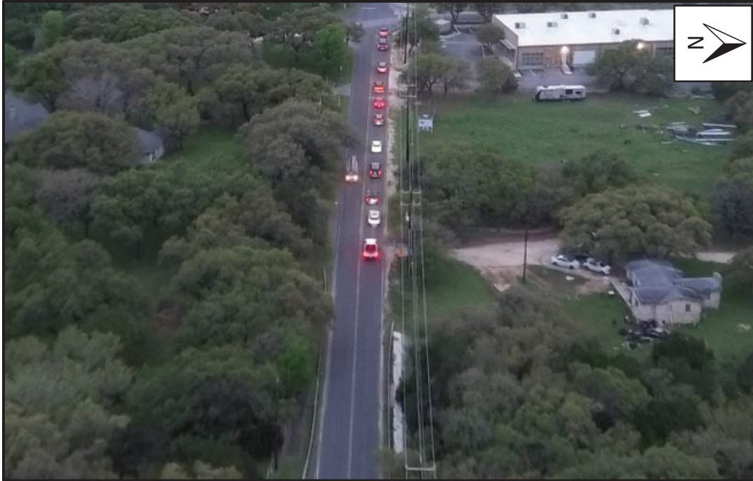
Figure 8 – Approximately 415 LF Queue at Dietz Elkhorn Rd and Old Fredericksburg Rd (AM)
