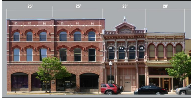
Figure 7-3 6.6 Illustration showing building articulation requirement
