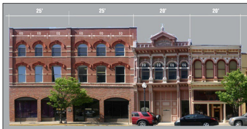
Figure 7-3 Illustration showing building articulation requirement
