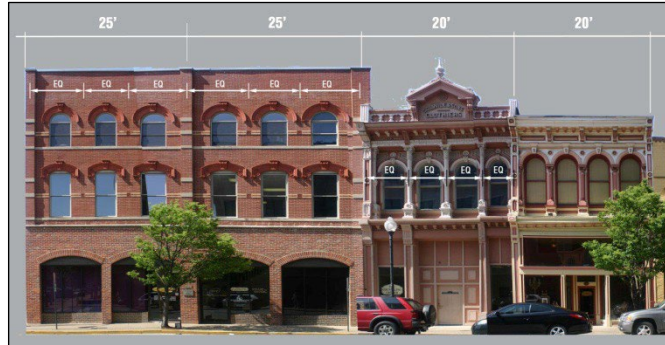
Figure 7-3 Illustration showing building articulation requirement
