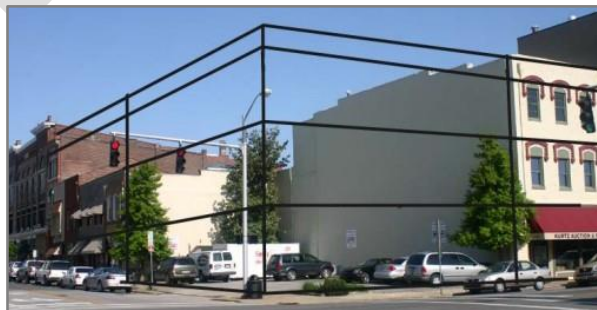
Figure 7-5 Figure showing how horizontal elements should match in the design of infill buildings.
