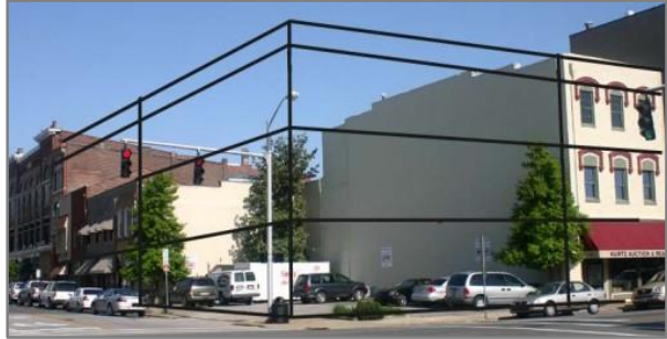
Figure 7-5-6.8 Figure showing how horizontal elements should match in the design of infill buildings.
