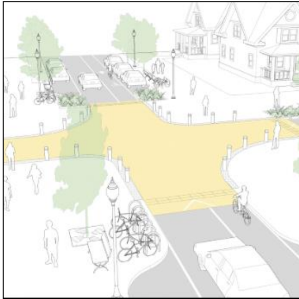
Picture 2: Raised Intersection
