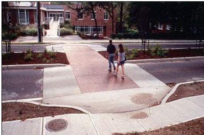
Picture 1: Raised Crosswalk speed reduction
