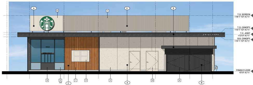
4 SOUTH ELEVATION SCALE: 3/16" = 1'-0"
