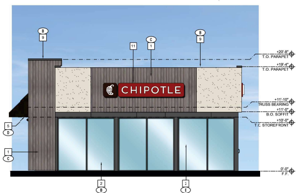
4 EAST ELEVATION SCALE: 3/16" = 1'-0"
