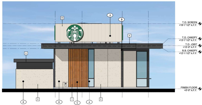
2 EAST ELEVATION SCALE: 3/16" = 1'-0"
