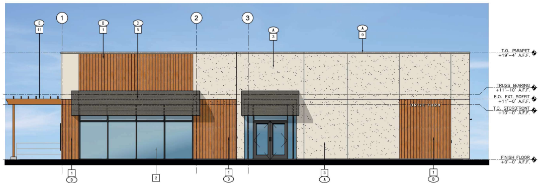
3 WEST ELEVATION SCALE: 3/16" = 1'-0"
