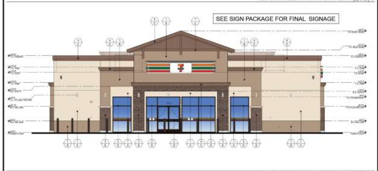
EXTERIOR ELEVATION - SOUTHEAST SCALE 1/8" = 1'-0" 1
