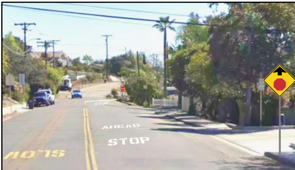
Figure 11. “STOP AHEAD” (W3-1) Warning Signs and Pavement Legends on Juniper Street.
