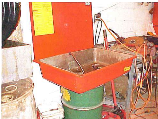
Solvent-based parts washer: The spent solvent must be picked up by an authorized hazardous waste transporter.
