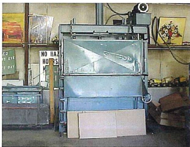
Aqueous (water based) parts washer: These units typically use the same water over and over again, and therefore can reduce the amount of hazardous waste generated by washing parts. Even so, the accumulated sludge must be handled as a hazardous waste, unless laboratory test results show it is non-hazardous.
