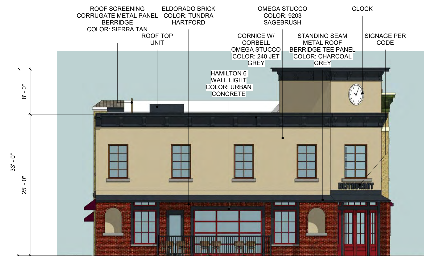
2 BUILDING 1 - SIDE ELEVATION 1 1/8" = 1'-0"
